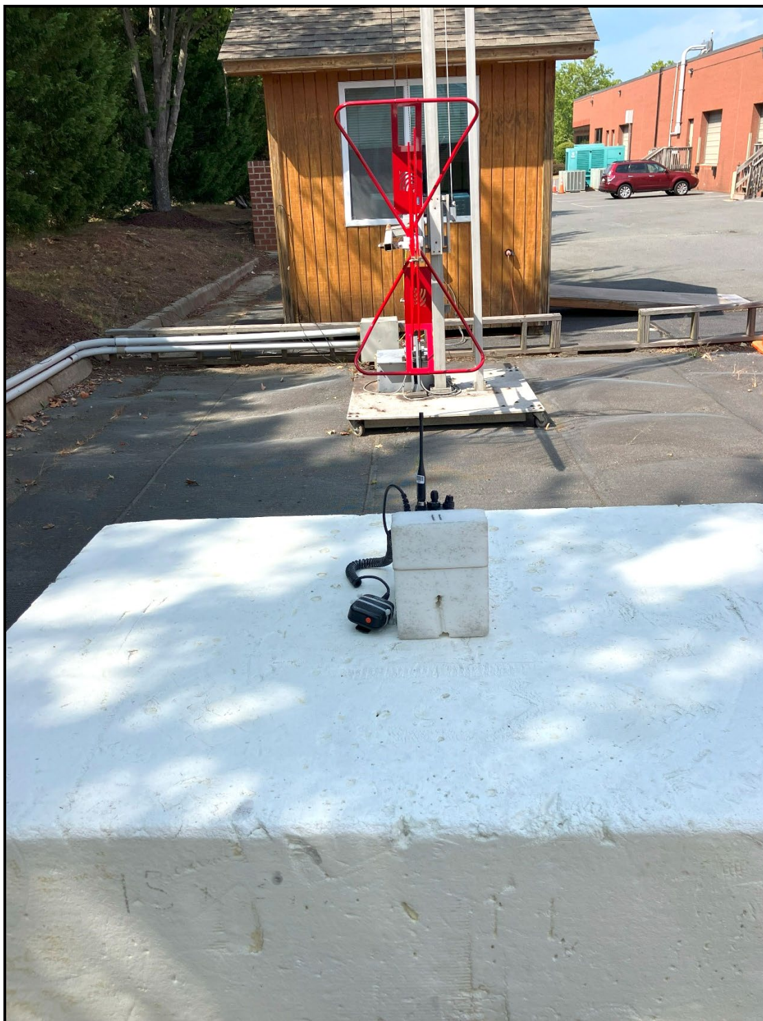
Photograph 4: Radiated Emissions (Spurious/Harmonics) Under 1 GHz, Back View
