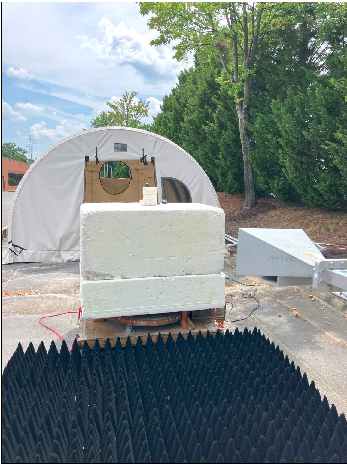
Photograph 2: Radiated Emissions (Spurious/Harmonics) Over 1 GHz, Back View
