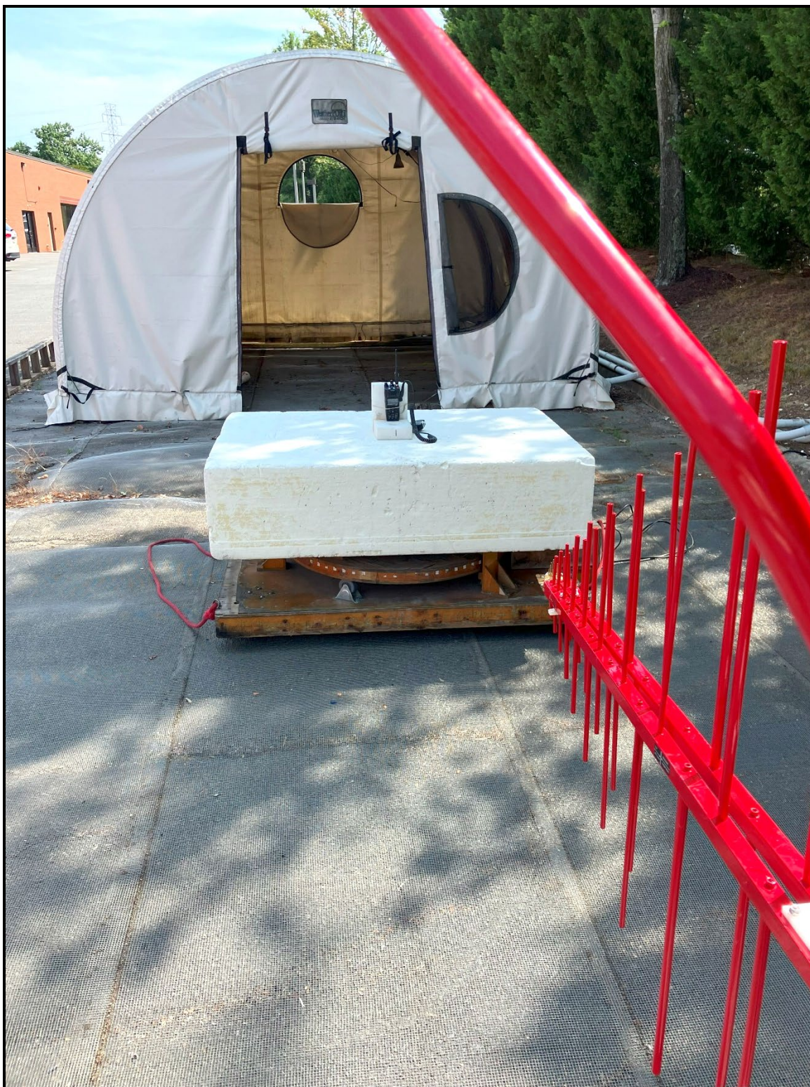
Photograph 3: Radiated Emissions (Spurious/Harmonics) Under 1 GHz, Front View
