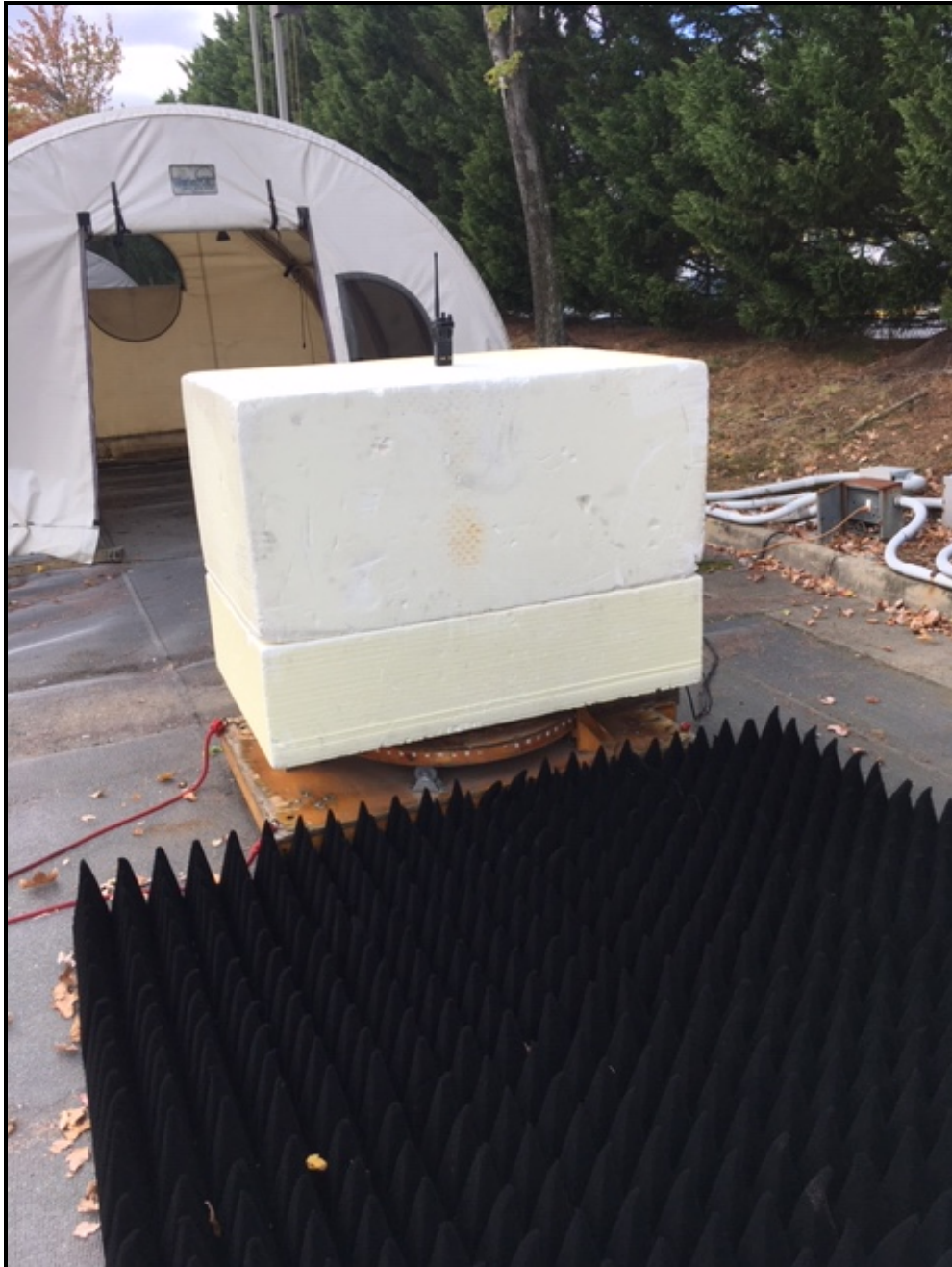
Photograph 2: Radiated Emissions (Spurious/Harmonics) Over 1 GHz, Back View
