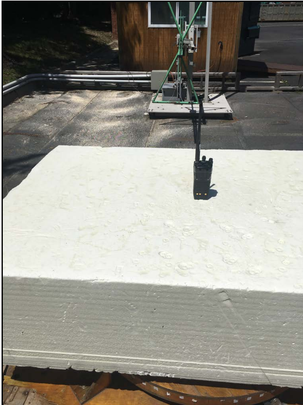
Photograph 4: Radiated Emissions (Spurious/Harmonics) Under 1 GHz, Back View
