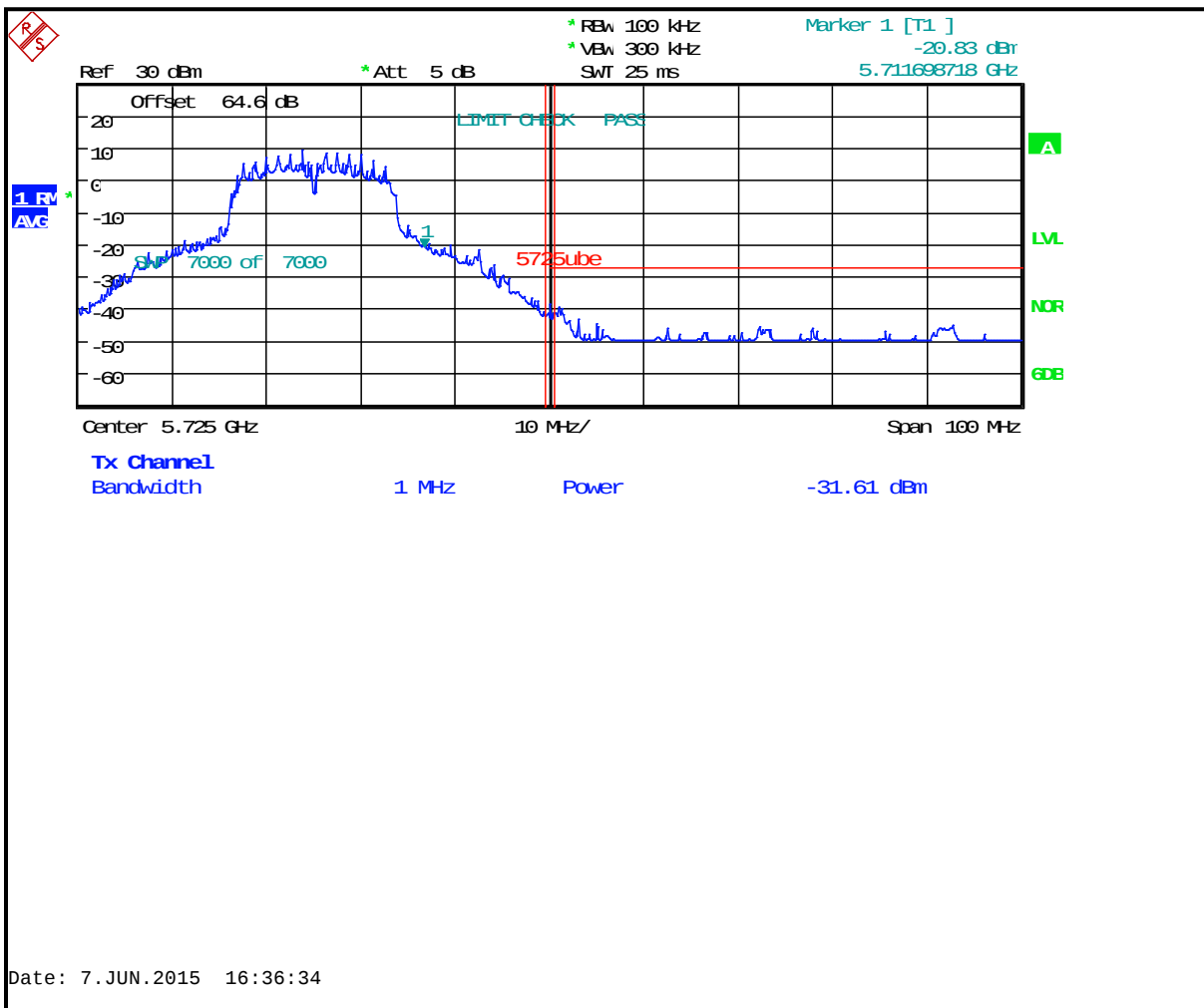
Plot 6-28: Upper Band Edge: Measurement Channel 140 (5700 MHz, 802.11n, Average)
