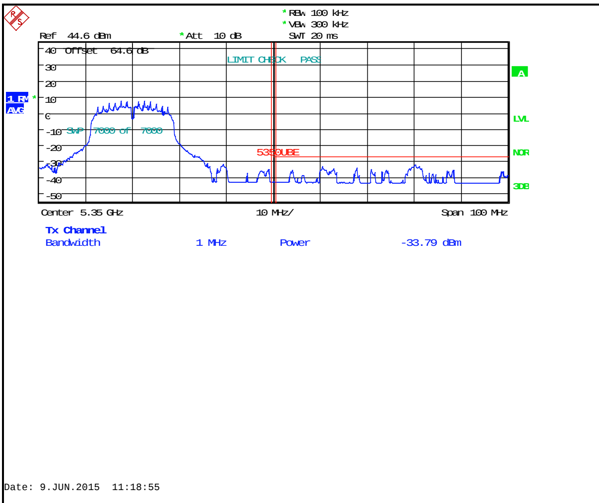
Plot 6-10: Upper Band Edge: Measurement Channel 64 (5320 MHz, 802.11a, Average)
