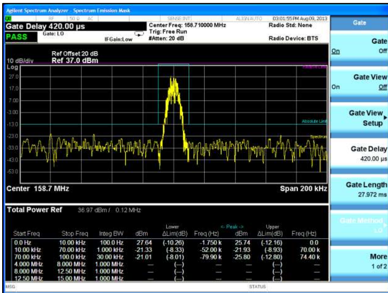
Plot 7-54: Occupied Bandwidth – 158.710 MHz; Mask; H-CPM TDMA
