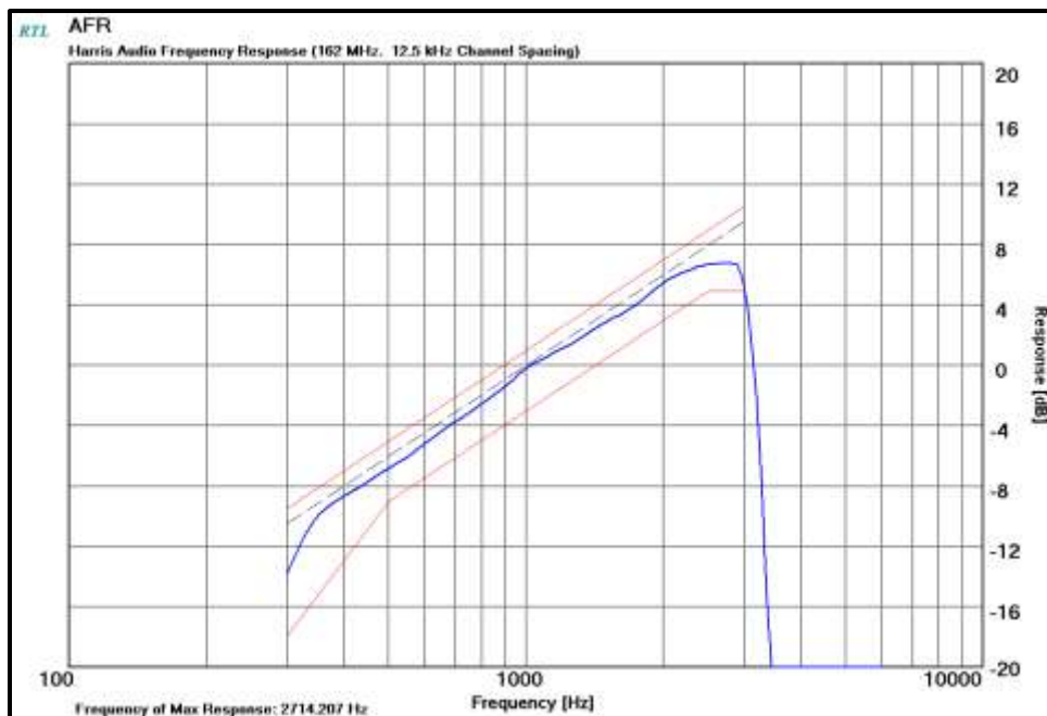
Plot 9-1: Modulation Characteristics - Audio Frequency Response – 162.0000 MHz
