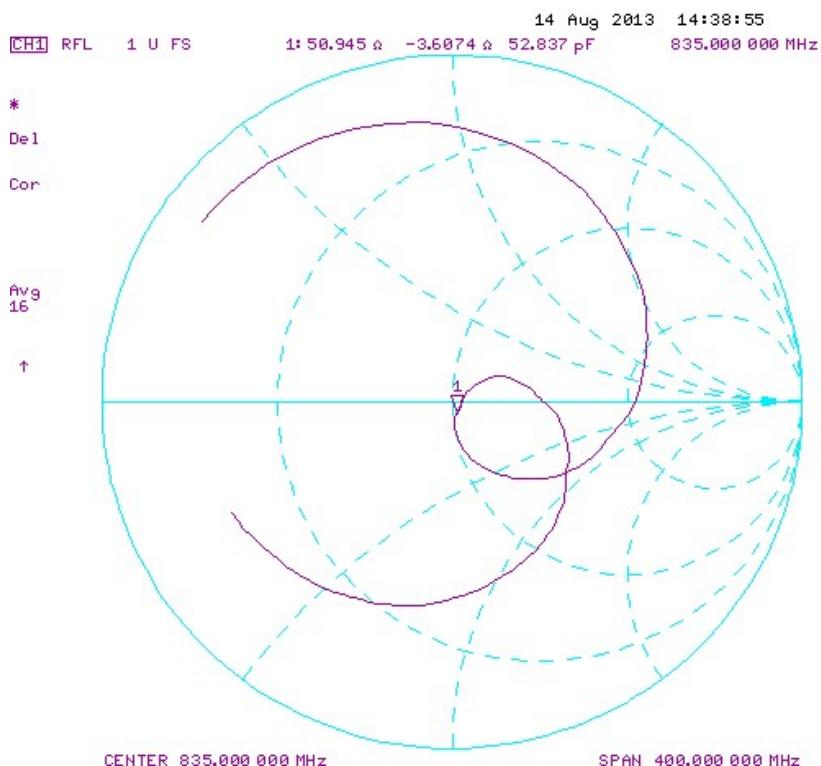
**835 MHz Dipole Extended Calibration****Antenna VSWR with Body TSL**
