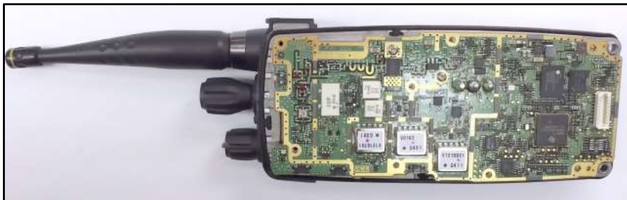
Photograph 15: Main PWB in Unit
