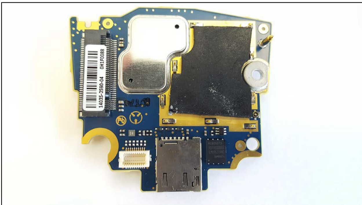
Expansion Board with LTE Processor Shield – Top
