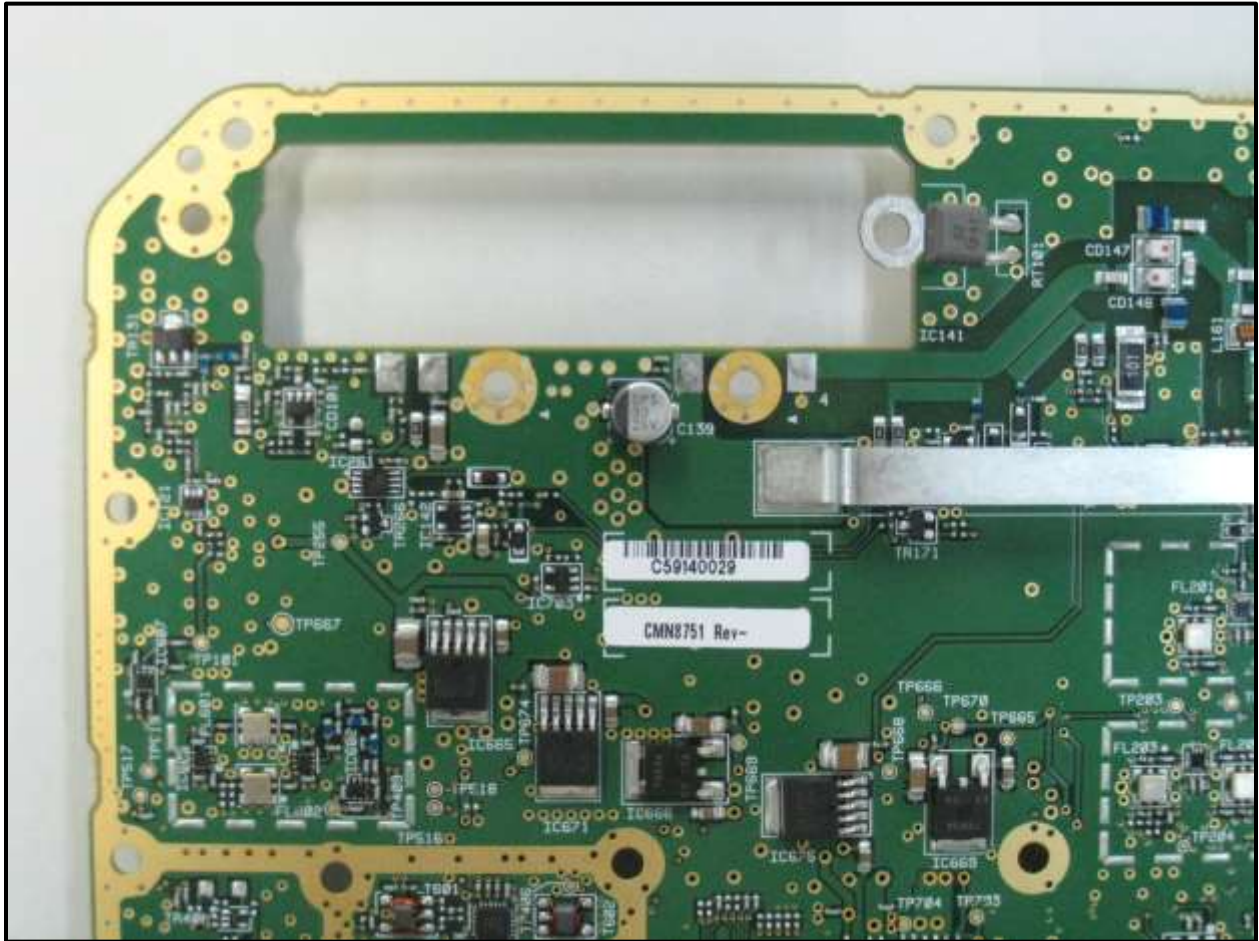
Photograph 22: RF Processor – Component Side; Upper Left
