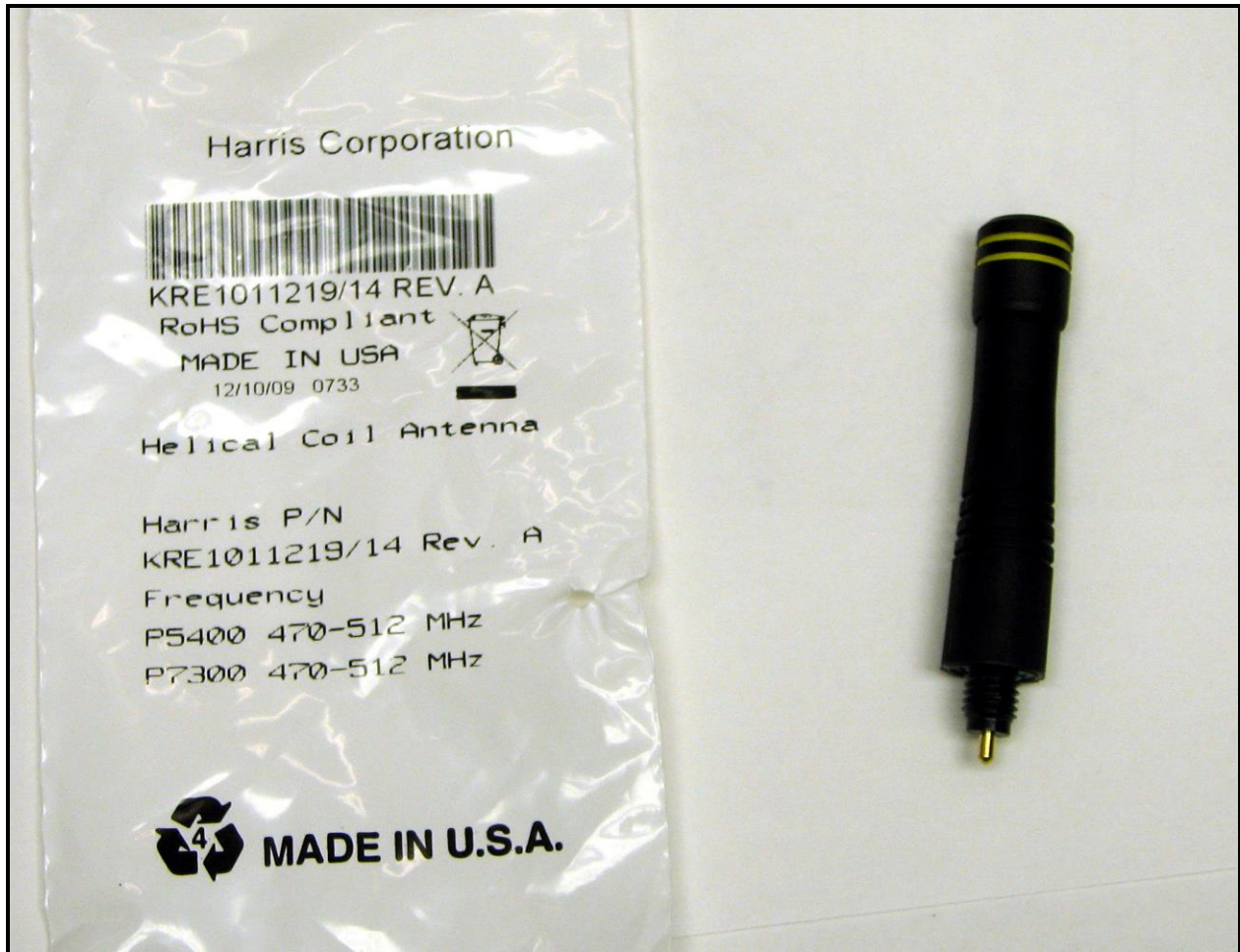
Photograph 20: Antenna Part # KRE 101 1219/14
