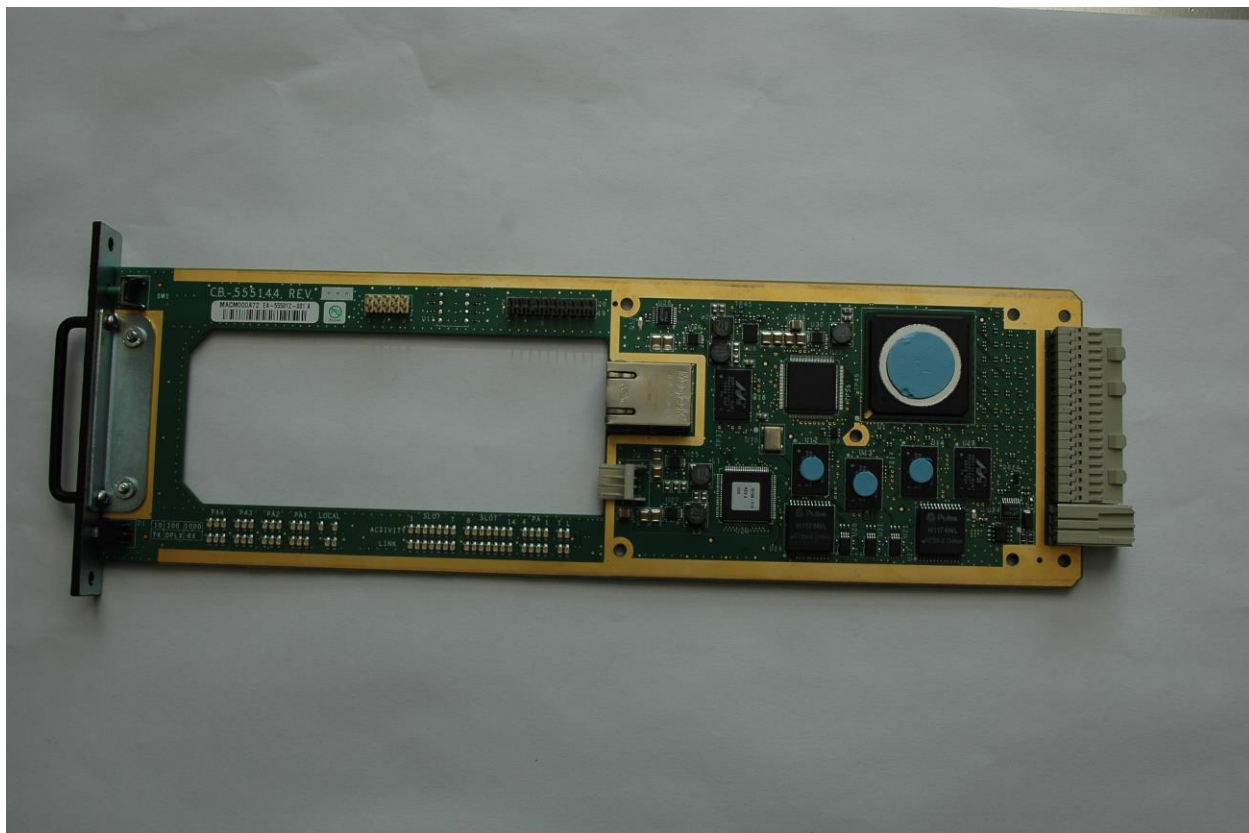
Photograph 6. E-Switch - Top Side
