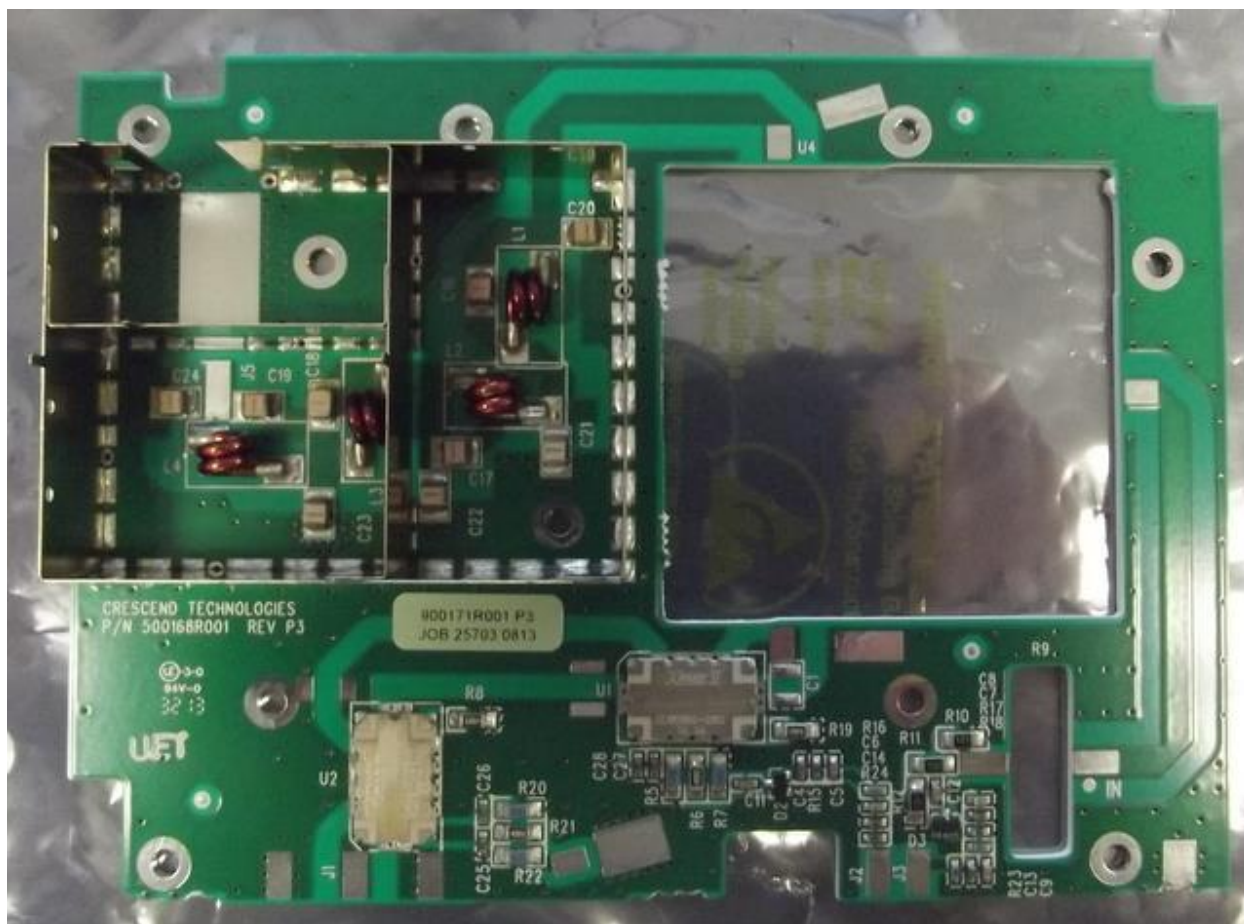
Photograph 15. Power Amplifier Output Assembly Top
