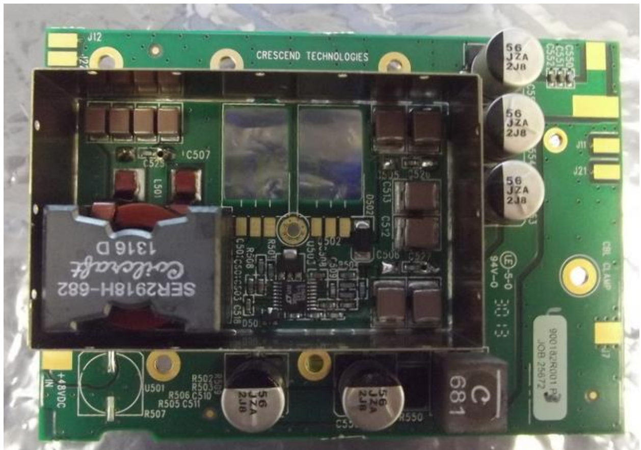
Photograph 17. Power Amplifier Switcher Assembly Top
