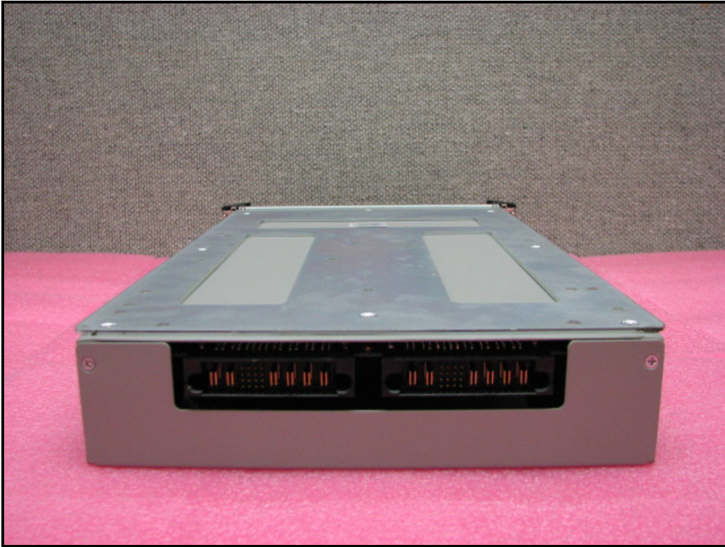
Photograph 12: Power Supply – Back View
