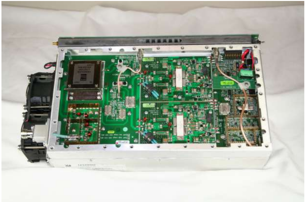
Photograph 1. HPA & Linearizer (470-520MHz) Top
