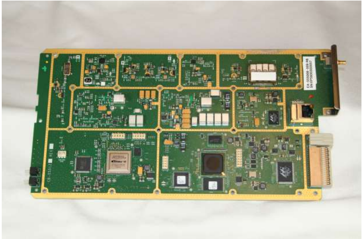
Photograph 8. TX Module (470-494MHz) Top
