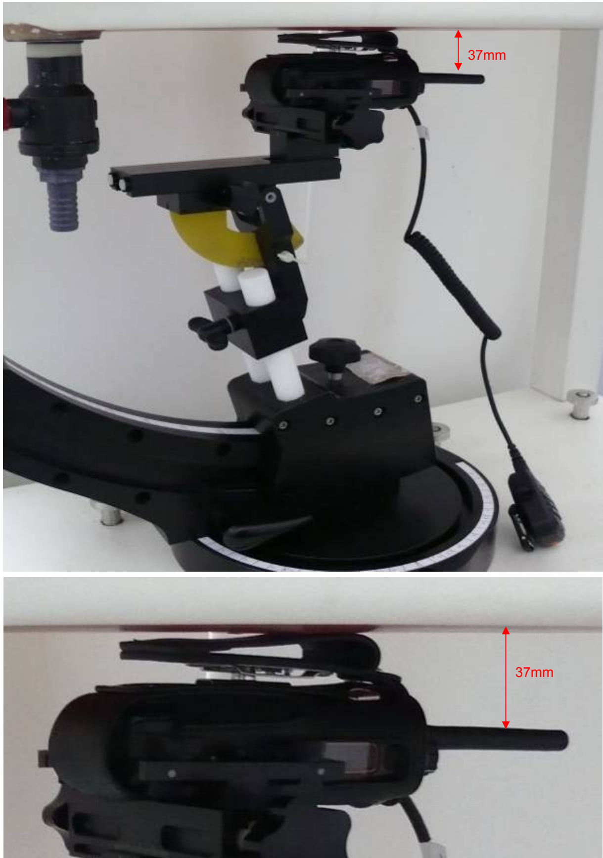
Picture 14: Body-worn with Thinner Battery, Pocket, Leather and Accessory 1, the front of the EUT towards ground, the distance from EUT Antenna to the bottom of the Phantom is 37mm
