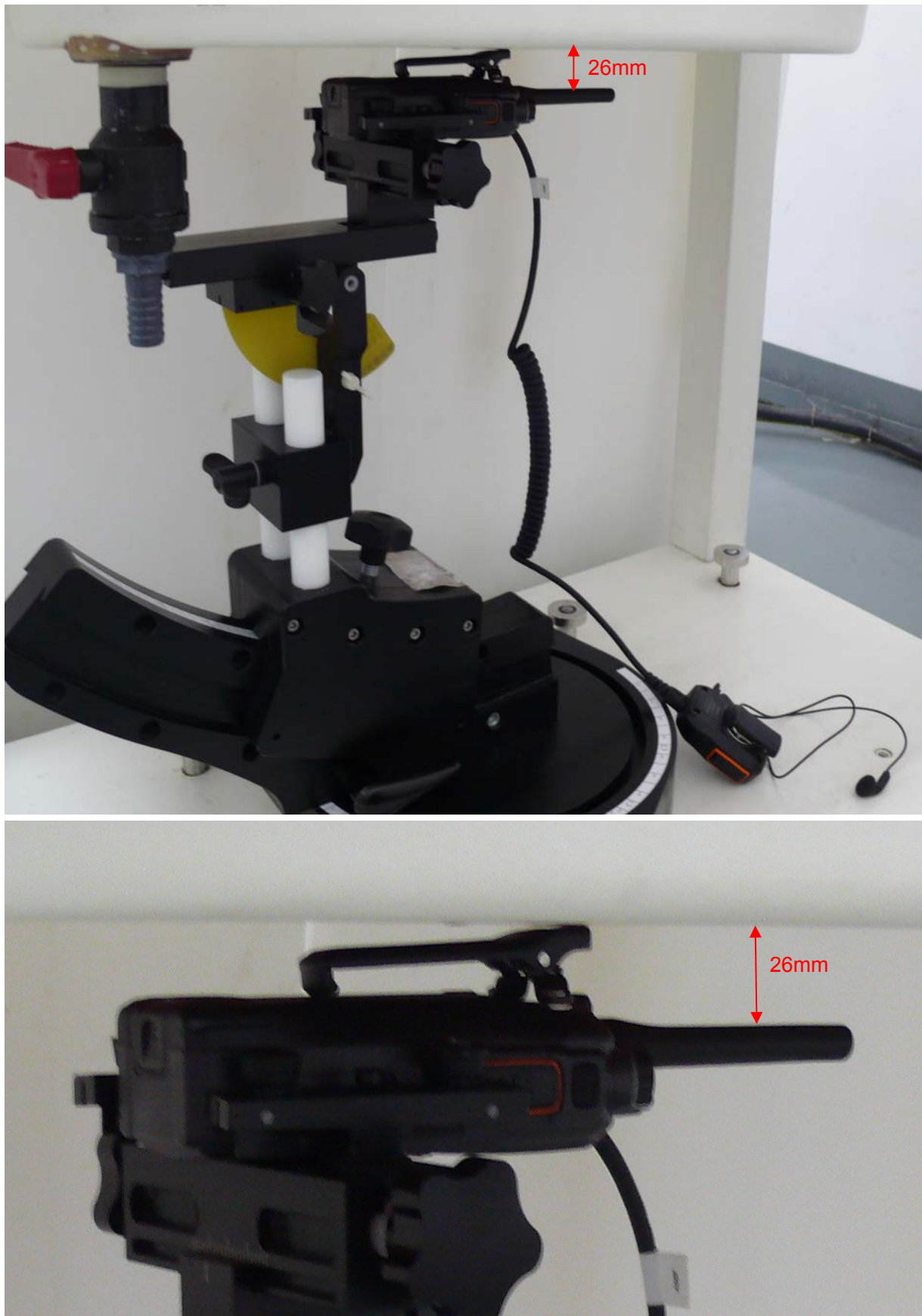
Picture 8: Body-worn with Thinner Battery, Belt, Accessory 1 and Earphone 2, the front of the EUT towards ground, the distance from EUT Antenna to the bottom of the Phantom is 26mm
