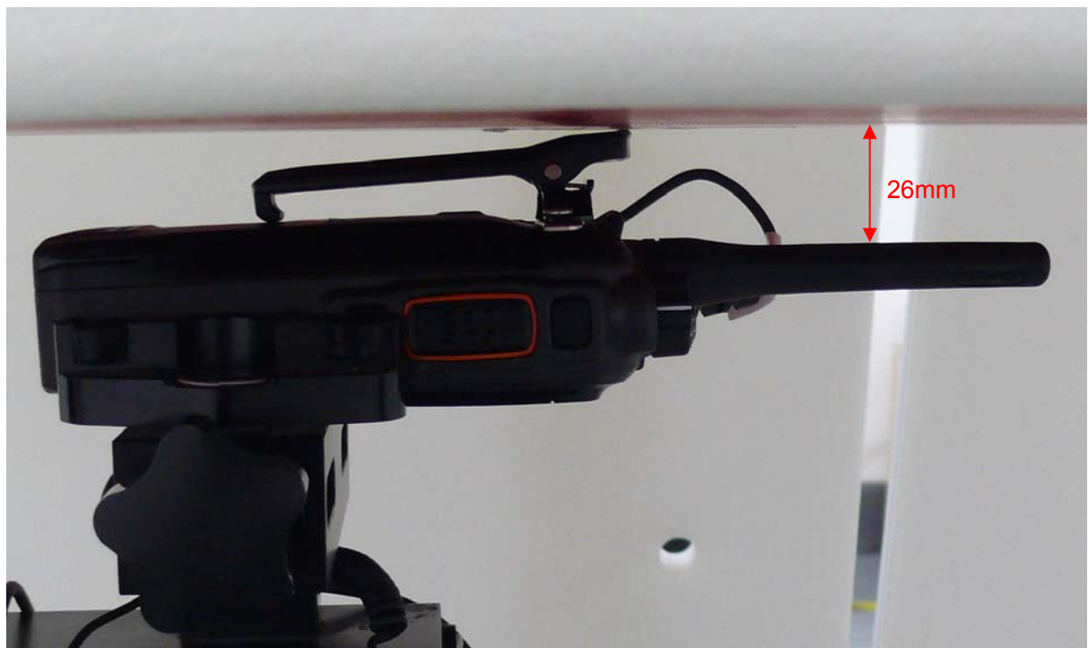
Picture 9: Body-worn with Thinner Battery, Belt and Audio Accessory 2, the front of the EUT towards ground, the distance from EUT Antenna to the bottom of the Phantom is 26mm
