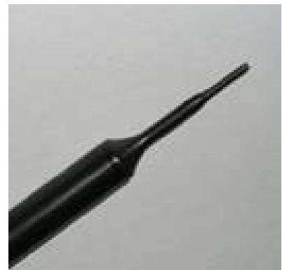
Figure 2. EX3DV4 E-field Probe
