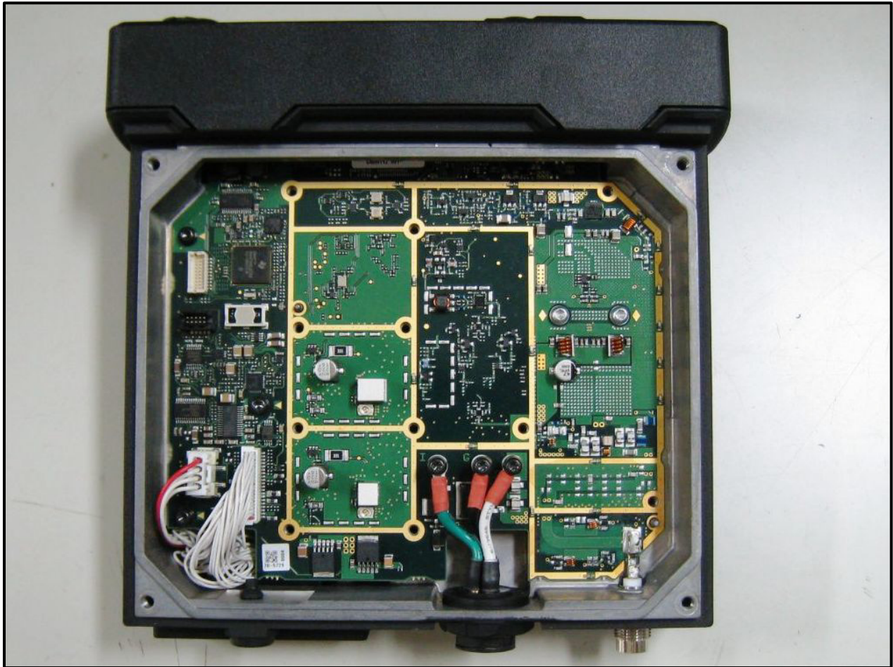
Photograph 14: Bottom Cover and Shield Removed
