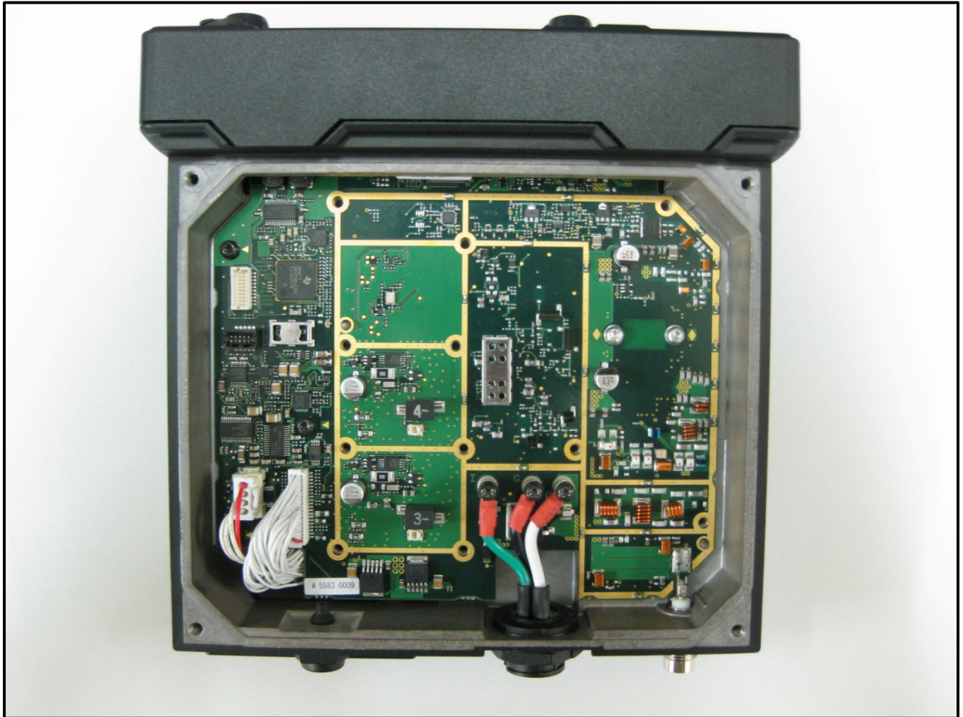
Photograph 14: Bottom Cover and Shield Removed
