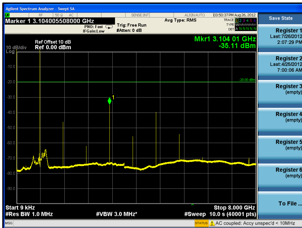
Plot 6-4: Spurious Emissions at Antenna Terminals – 794.0125 MHz
