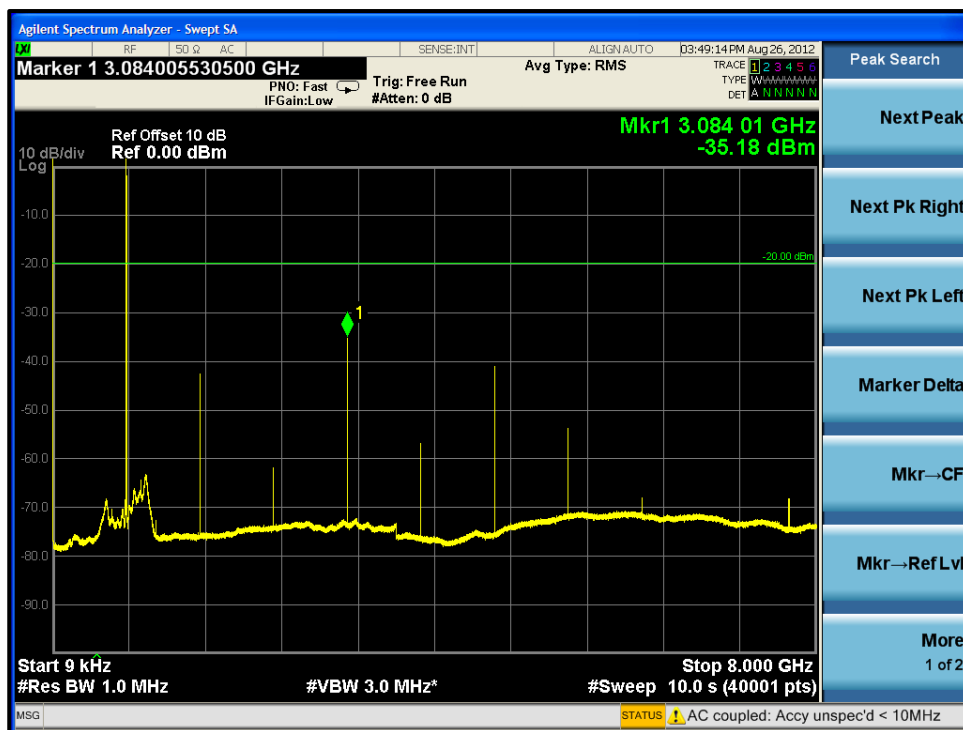
Plot 6-2: Spurious Emissions at Antenna Terminals – 771.00625 MHz
