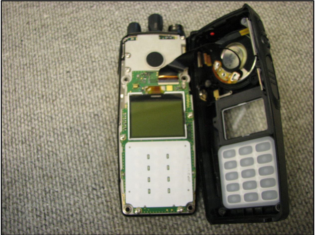
Photograph 12: Front Cover Removed
