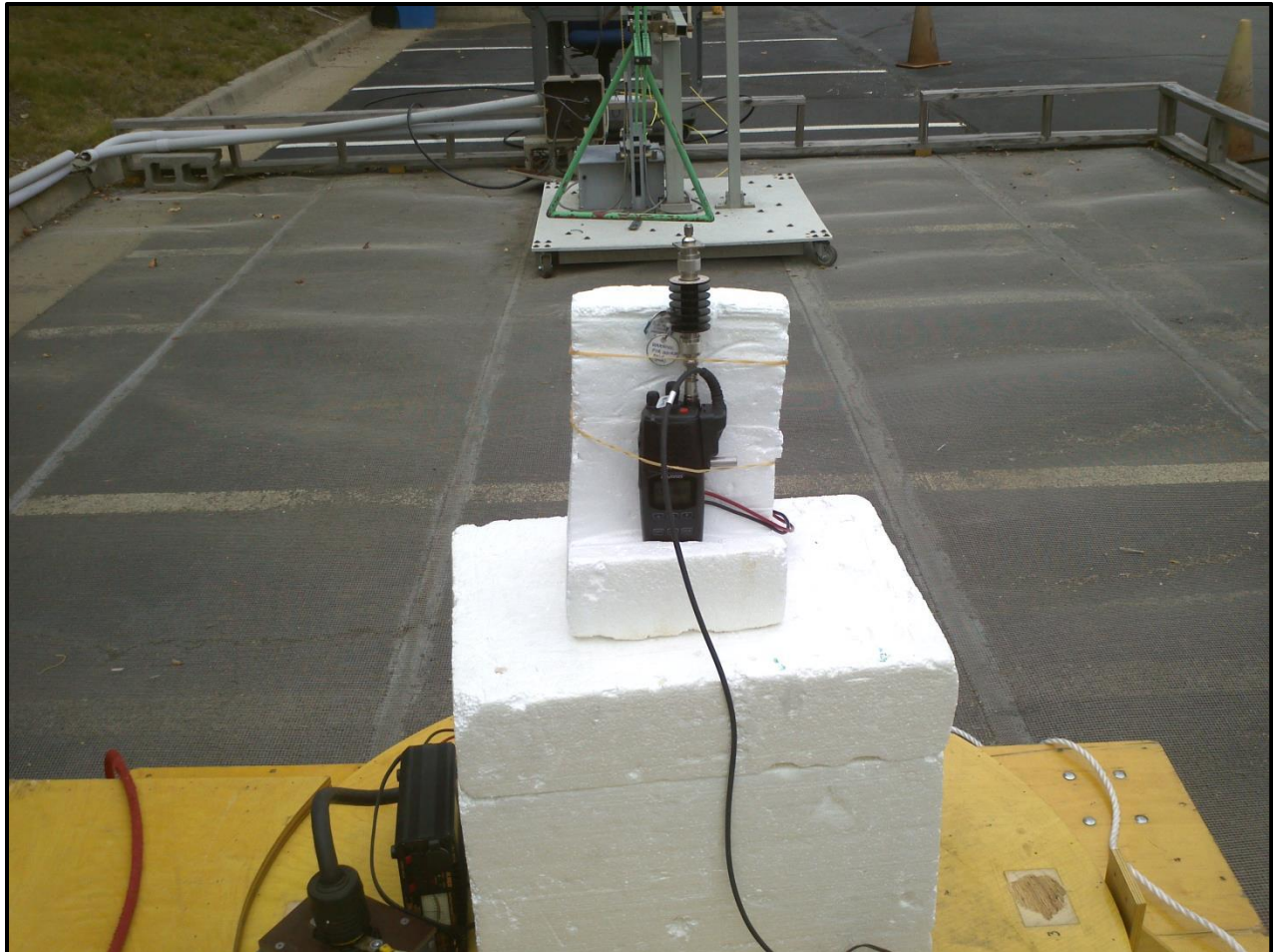
Photograph 1: Radiated TX Spurious Emissions – Front View
