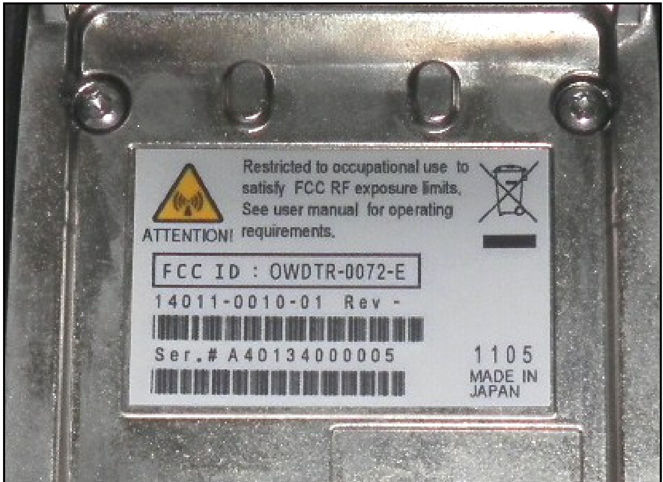
Photograph 3: RF Safety Label
