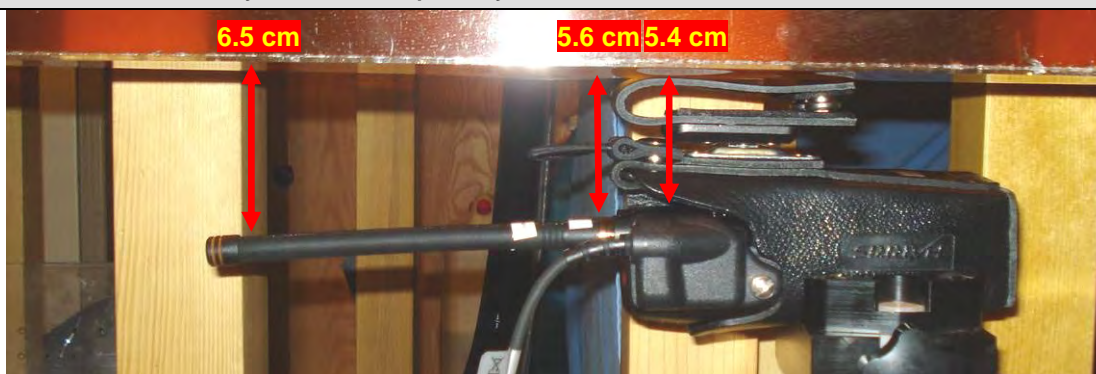
Body-worn Test Setup – Body-worn acc. 3, Audio acc. G7a, Antenna 1
