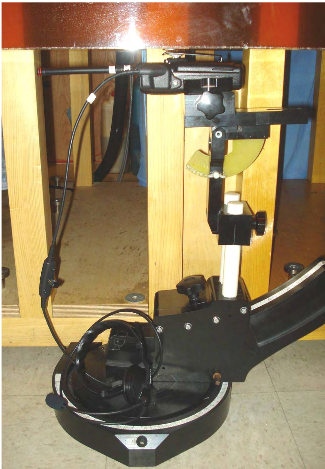
Body-worn Test Setup – Antenna 2, Body-worn Acc. 5, and Audio Acc. G2
