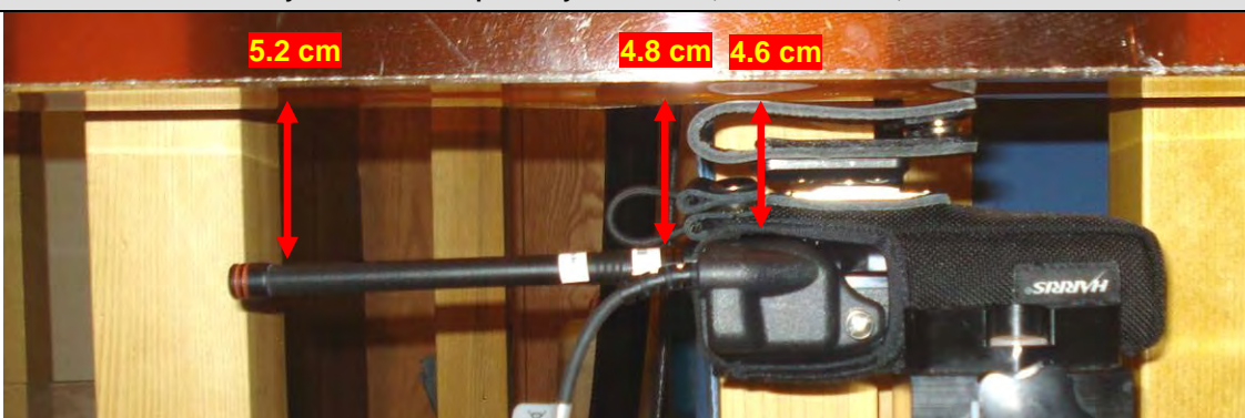
Body-worn Test Setup – Body-worn acc. 1, Audio acc. G47a Antenna 3
