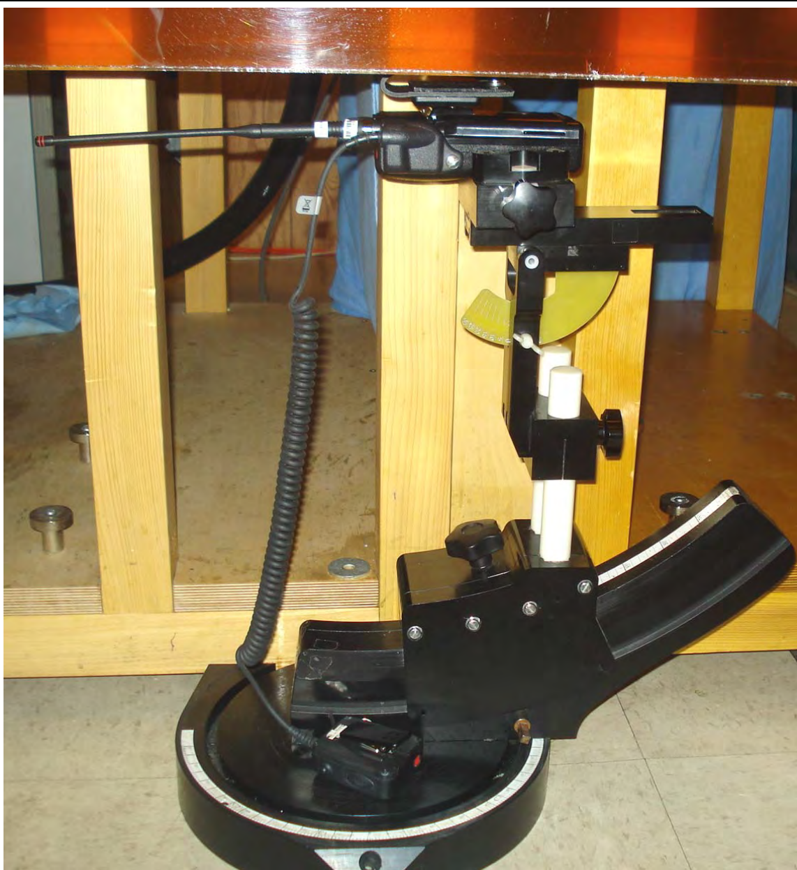
Body-worn Test Setup – Body-worn acc. 6, Audio acc. G7a, Antenna 4
