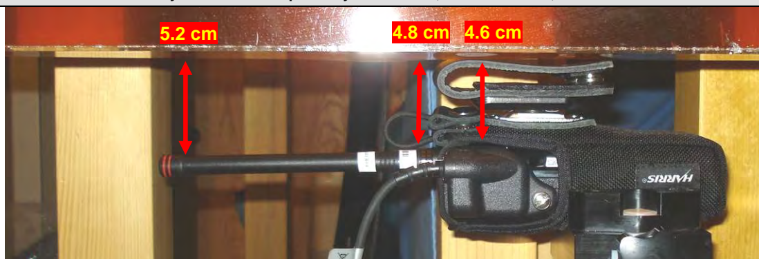
Body-worn Test Setup – Body-worn acc. 1, Audio acc. G7a, Antenna 2
