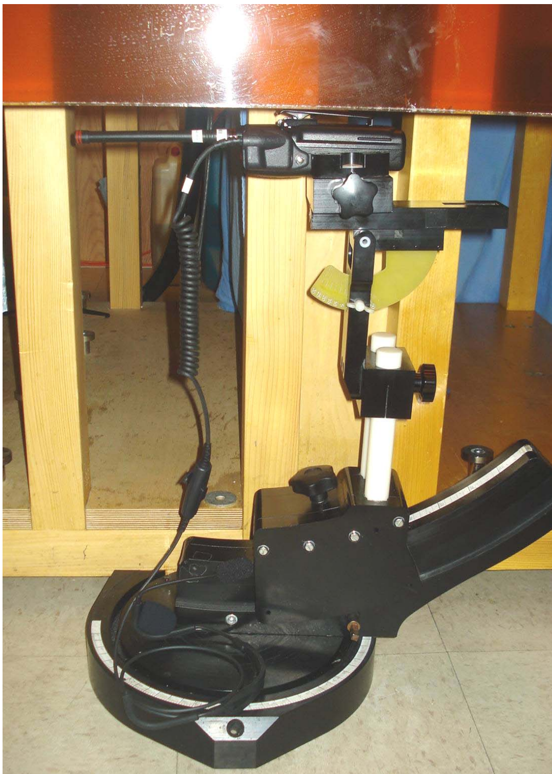
Body-worn Test Setup – Antenna 2, Body-worn Acc. 5, and Audio Acc. G5
