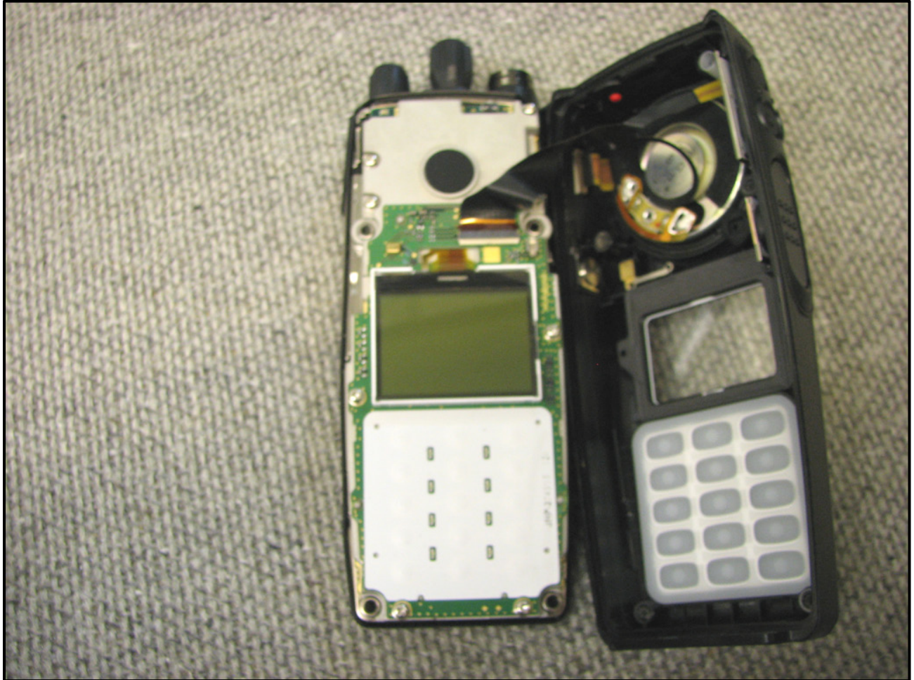
Photograph 14: Front Cover Removed
