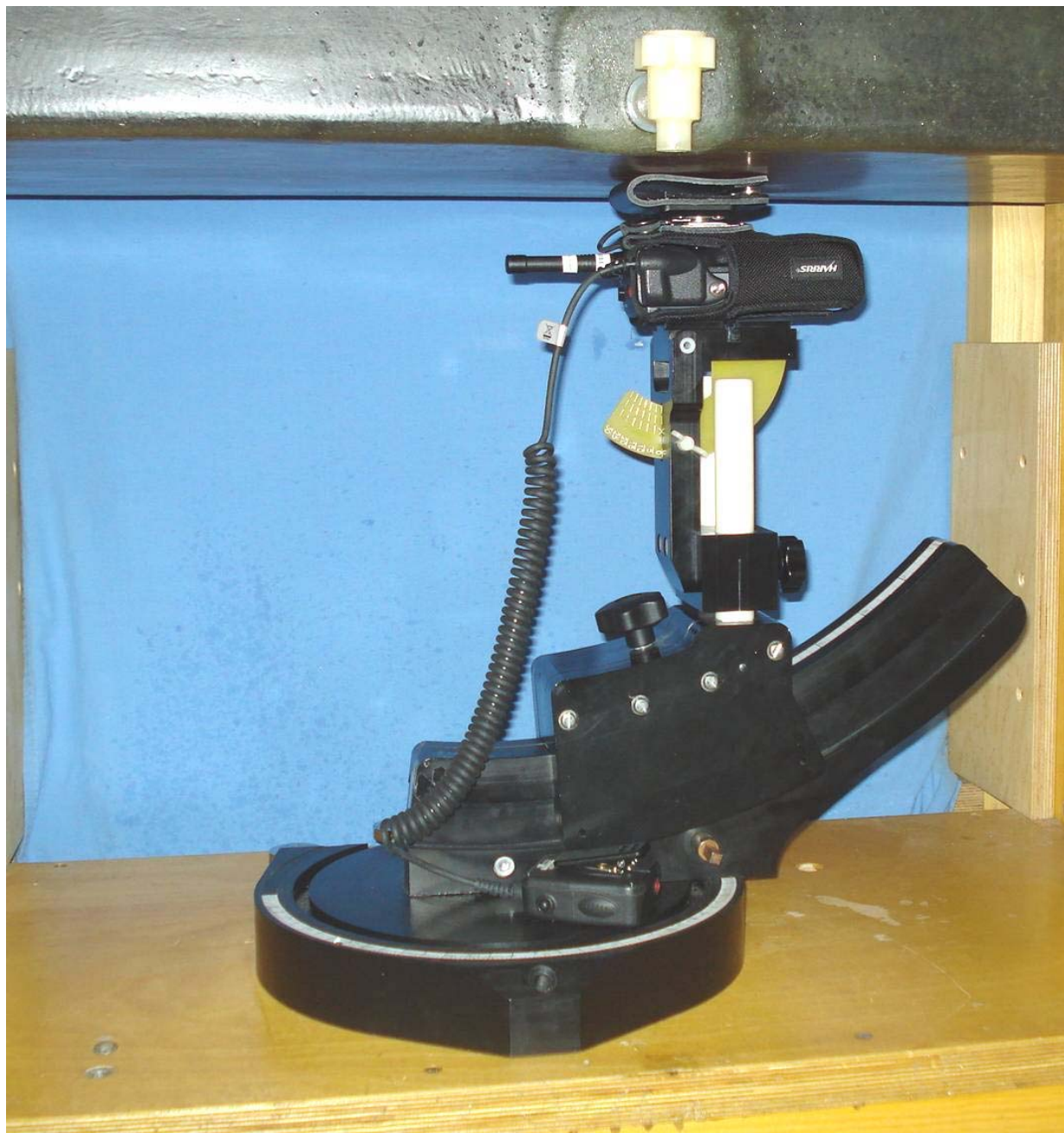
Body-worn test setup - DUT w/ Speaker-Mic (MC-023933-001), Nylon Case (14011-0012-01), Antenna 1 (KRE1011219/10)
