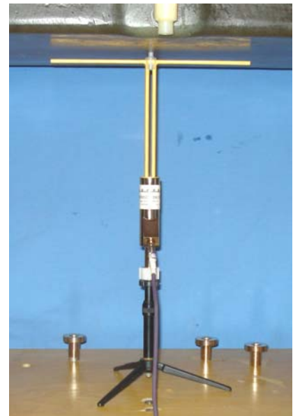
450 MHz SPEAG Validation Dipole Setup
