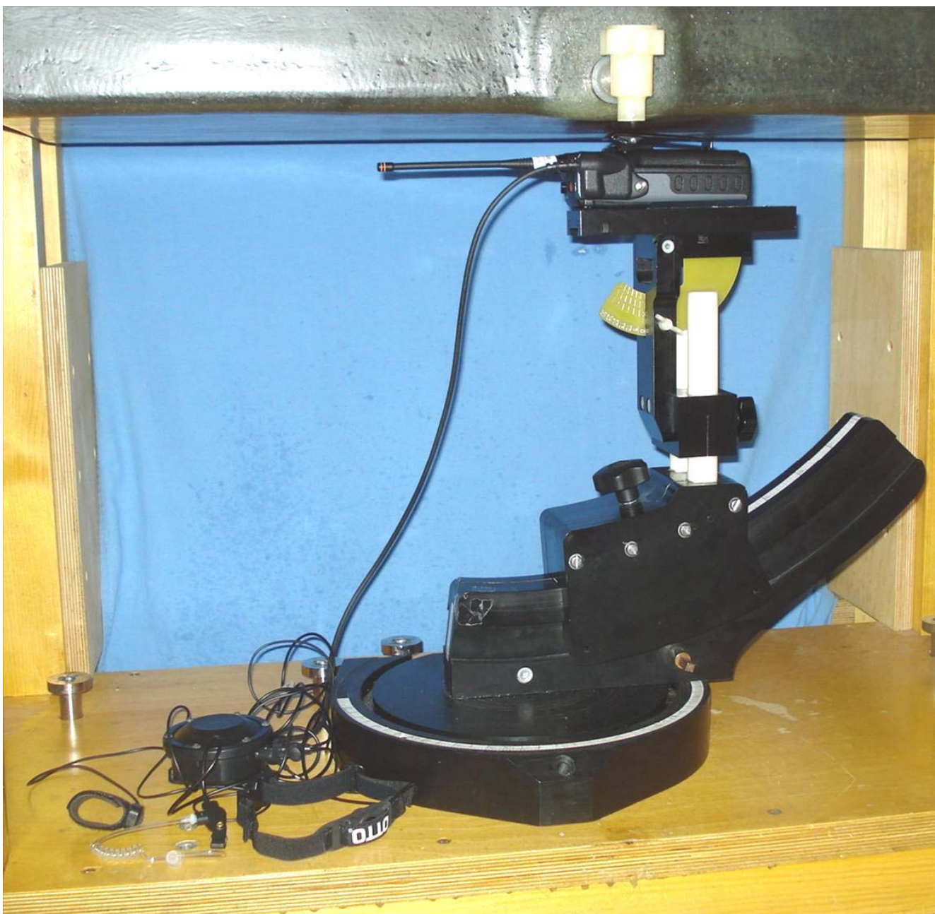
Body-worn test setup - DUT w/ Belt-clip (CC23894), Antenna 3 (KRE1011223/12), Audio Accessory G11b (EA-009580-015)
