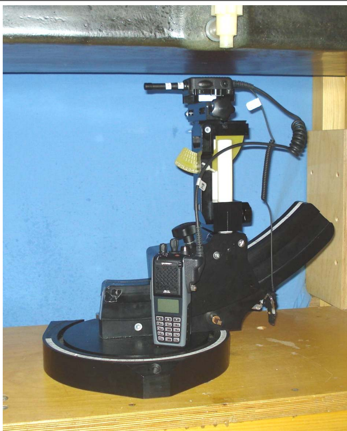
Speaker-Mic with Antenna (MC-023933-002) Face Held Test Setup Configuration
