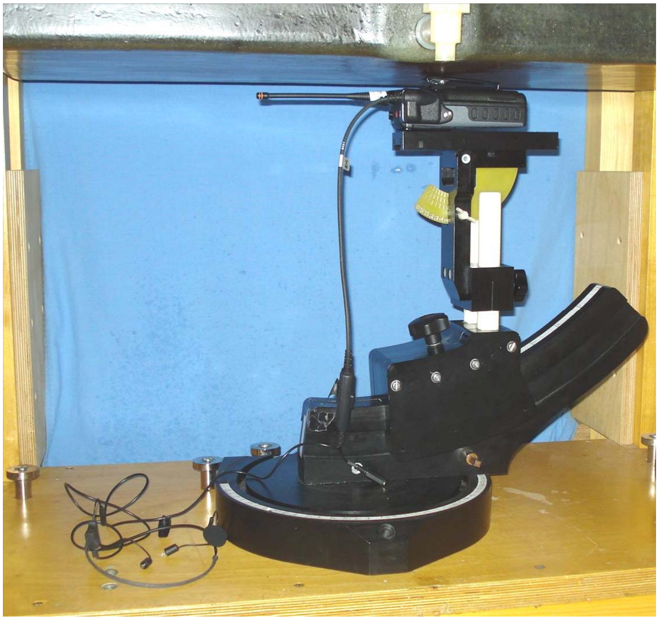
Body-worn test setup - DUT w/ Belt-clip (CC23894), Antenna 3 (KRE1011223/12), Audio Accessory G6b (EA-009580-018)
