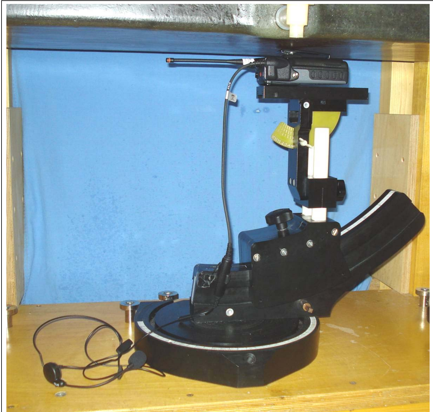
Body-worn test setup - DUT w/ Belt-clip (CC23894), Antenna 3 (KRE1011223/12), Audio Accessory G3b (EA-009580-016)
