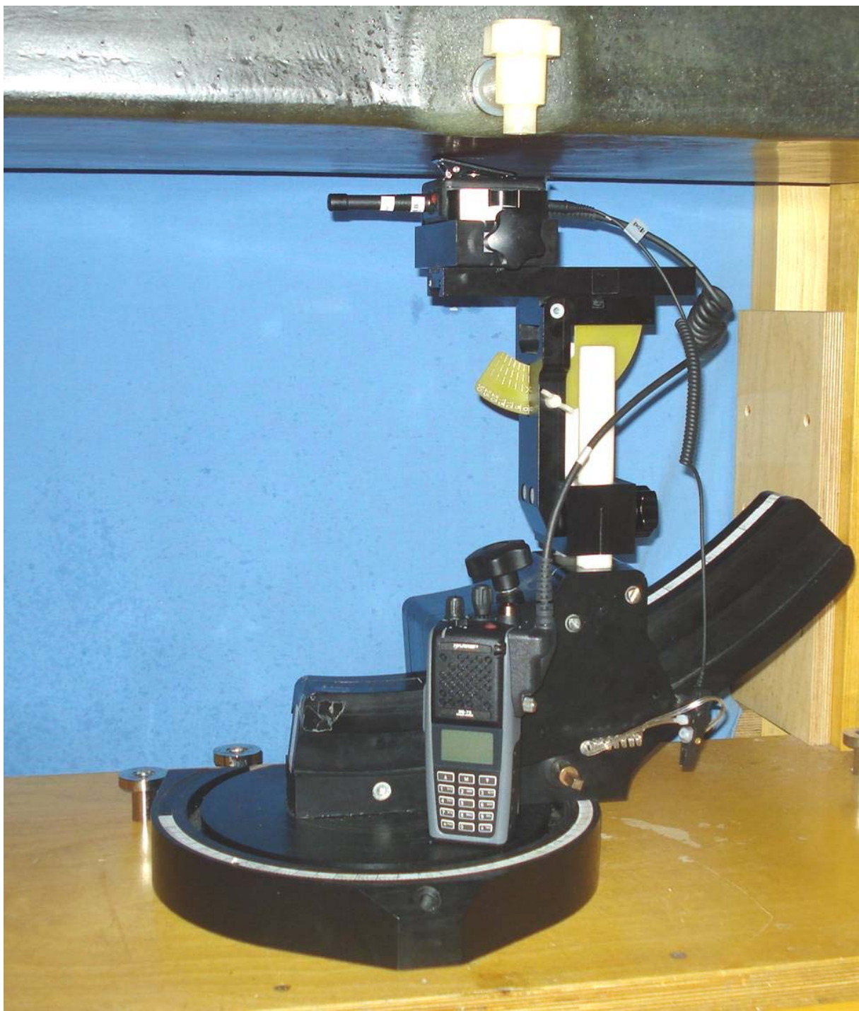
Speaker-Mic with Antenna (MC-023933-002) Body Worn Test Setup Configuration
