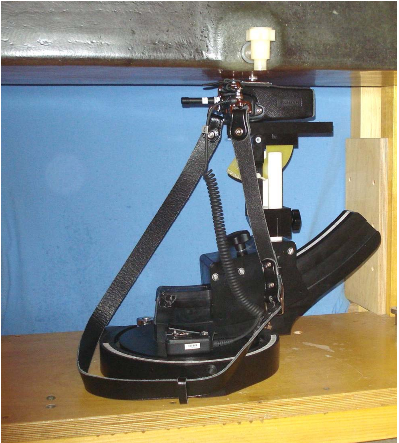
Body-worn test setup - DUT w/ Speaker-Mic (MC-023933-001), Leather Case w/ Shoulder Strap (14011-0012-04), Antenna 1 (KRE1011219/10)
