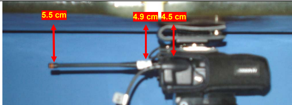
Body-worn test setup - DUT w/ Speaker-Mic (MC-023933-001), Nylon Case (14011-0012-01), Antenna 3 (KRE1011223/12)
