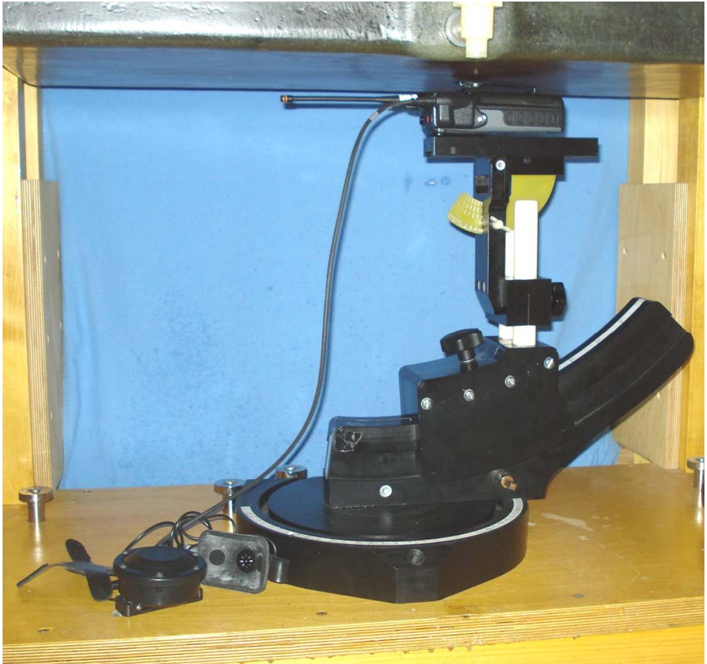
Body-worn test setup - DUT w/ Belt-clip (CC23894), Antenna 3 (KRE1011223/12), Audio Accessory G10 (EA-009580-012)
