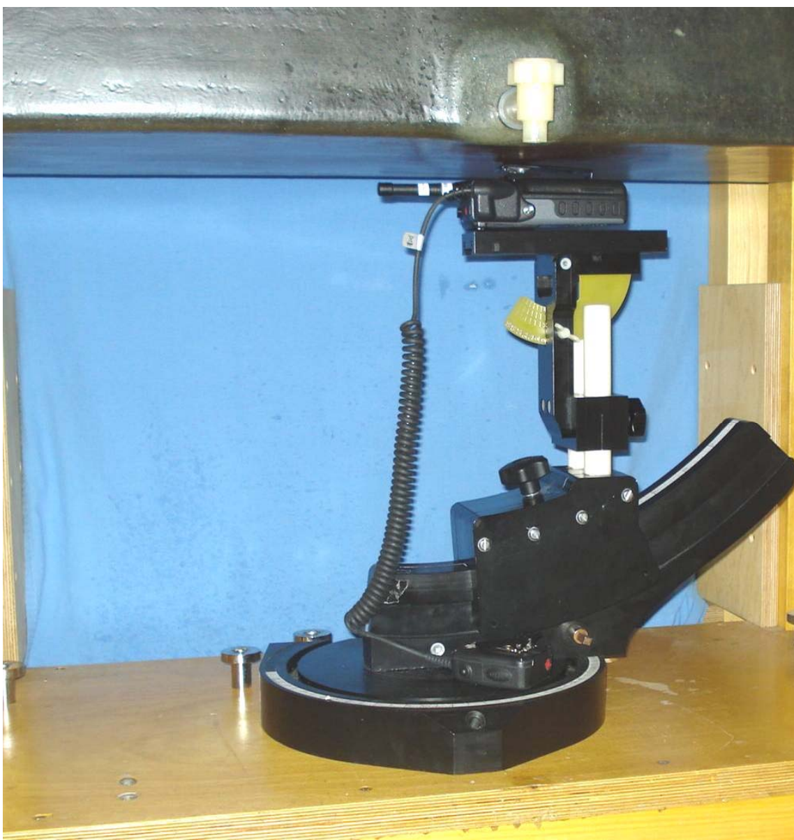
Body Worn Test Setup – DUT w/ Speaker-Mic (MC-023933-001), Belt-Clip (CC23894), Antenna 1 (KRE1011219/10)
