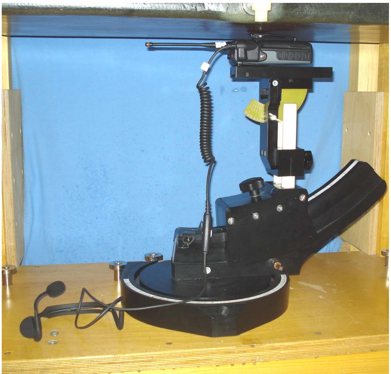
Body-worn test setup - DUT w/ Belt-clip (CC23894), Antenna 3 (KRE1011223/12), Audio Accessory G5 (EA-009580-011)
