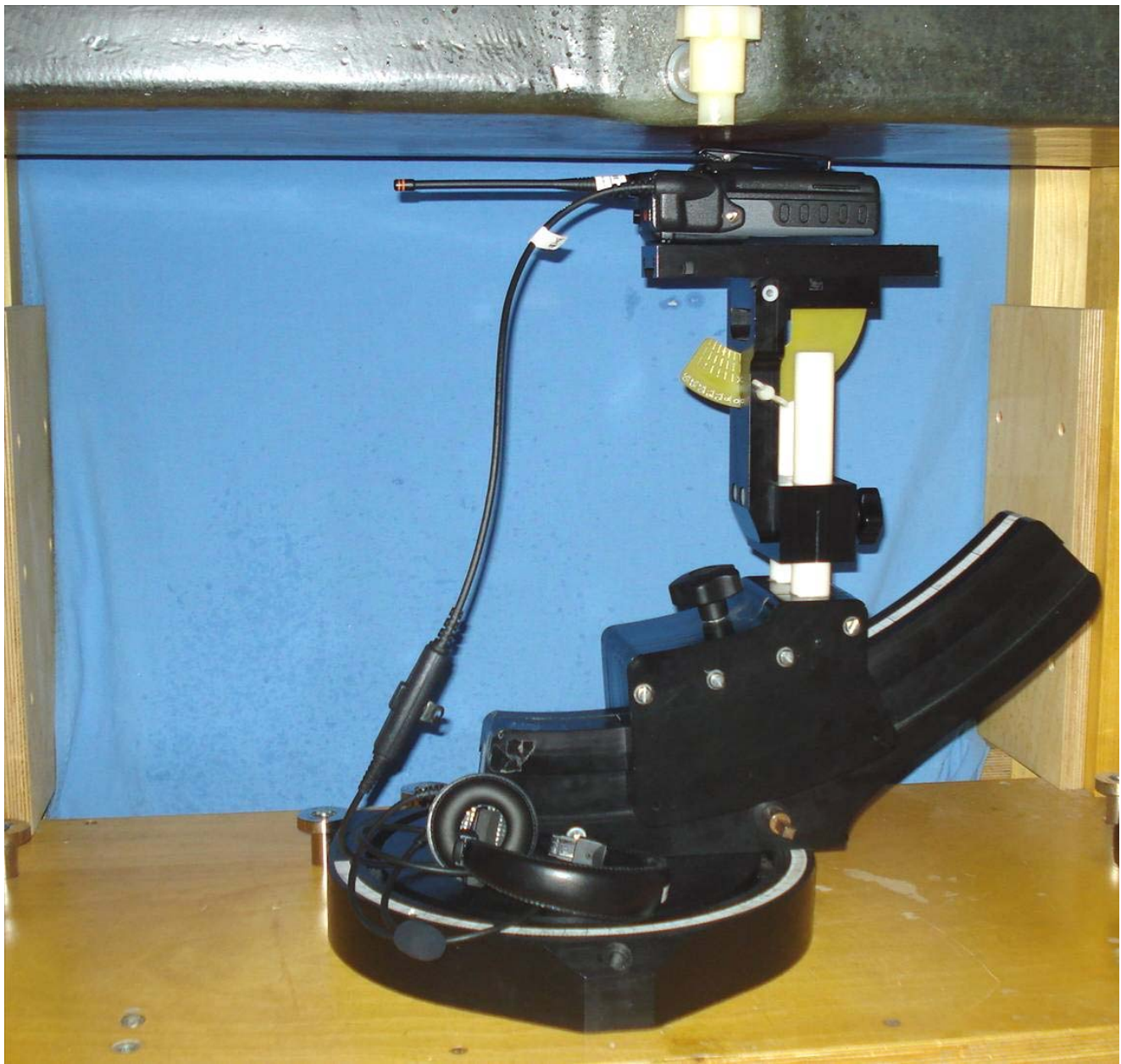
Body-worn test setup - DUT w/ Belt-clip (CC23894), Antenna 3 (KRE1011223/12), Audio Accessory G2 (EA-009580-008)
