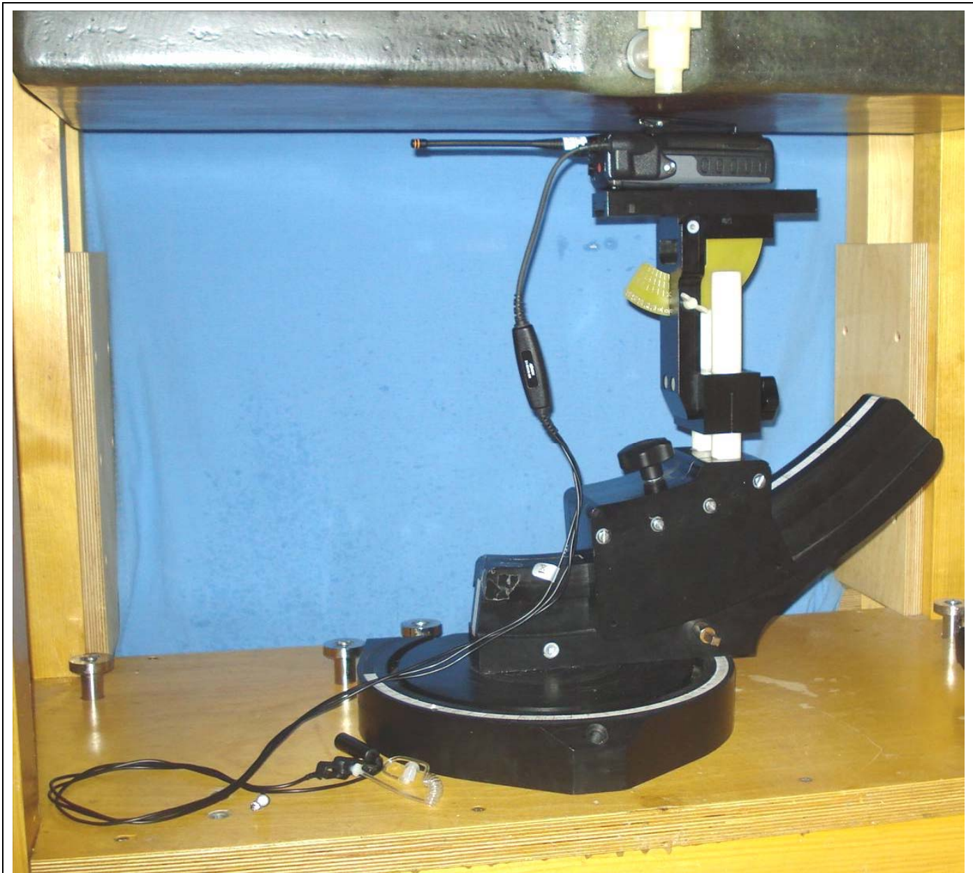
Body-worn test setup - DUT w/ Belt-clip (CC23894), Antenna 3 (KRE1011223/12), Audio Accessory G9a (EA-009580-005)
