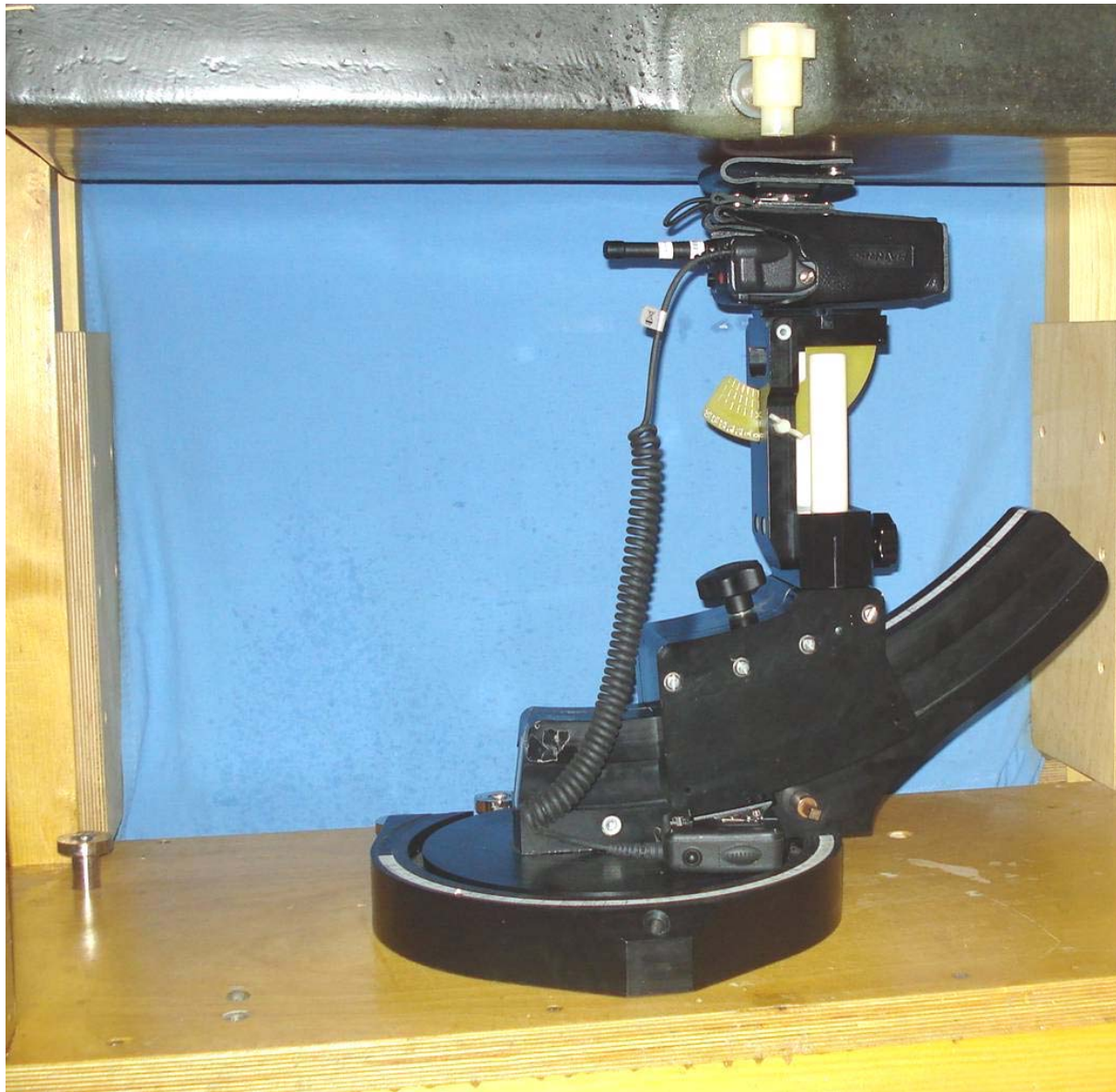
Body-worn test setup - DUT w/ Speaker-Mic (MC-023933-001), Leather Case (14011-0012-03), Antenna 1 (KRE1011219/10)
