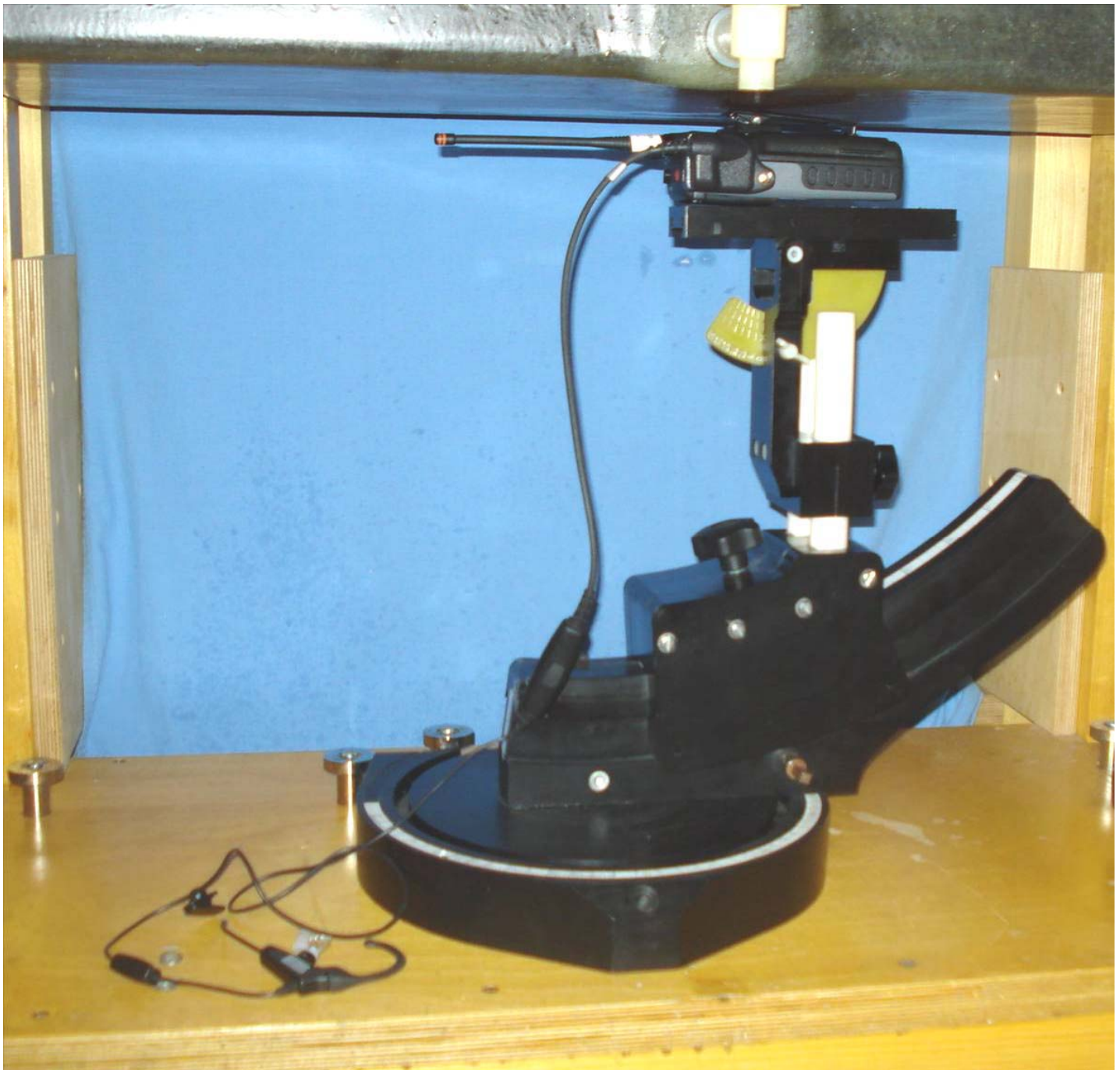
Body-worn test setup - DUT w/ Belt-clip (CC23894), Antenna 3 (KRE1011223/12), Audio Accessory G4 (EA-009580-007)
