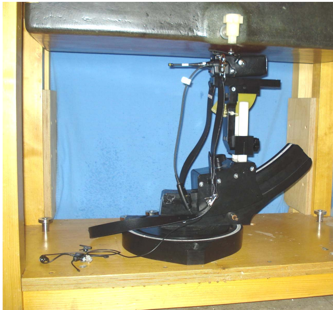
Body Worn Test Setup - Explorer Headset (EA-009580-007), Case (CC-023931-002), Antenna 1 (KRE1011223/01)
