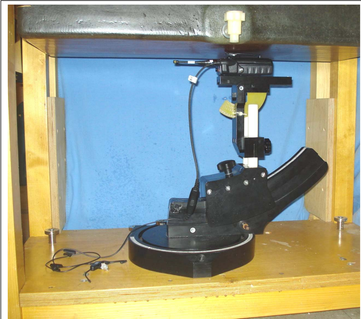
Body Worn Test Setup - Explorer Headset (EA-009580-007), Belt-Clip (CC23894), Antenna 1 (KRE1011223/01)
