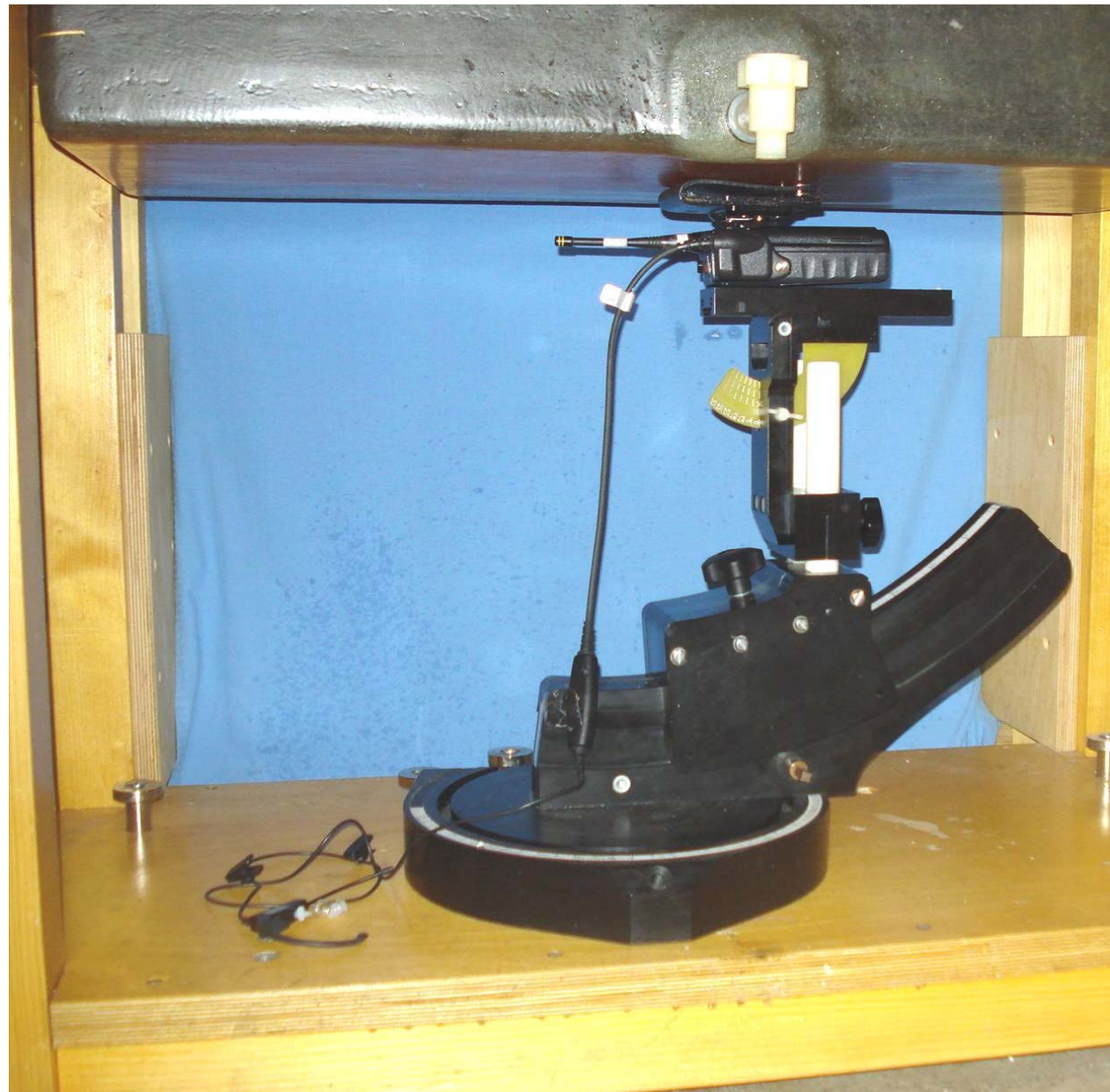
Body Worn Test Setup - Explorer Headset (EA-009580-007), Belt-Loop (KRY1011608/2), Antenna 1 (KRE1011223/01)
