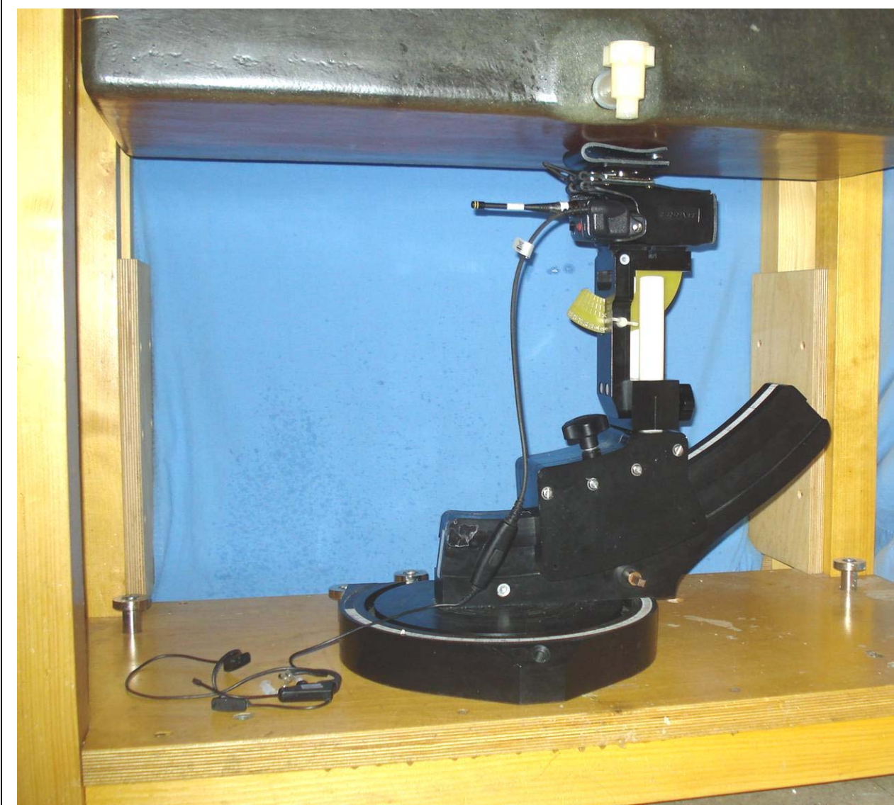
Body Worn Test Setup - Explorer Headset (EA-009580-007), Case (CC-014528-003), Antenna 1 (KRE1011223/01)
