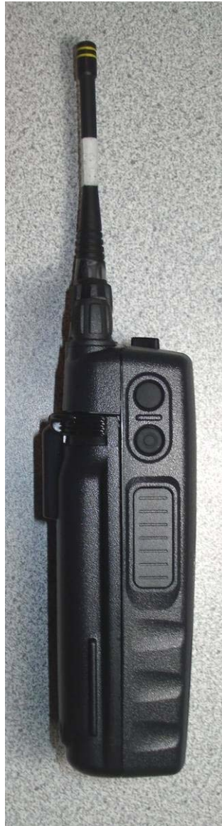
System Radio Left Side
