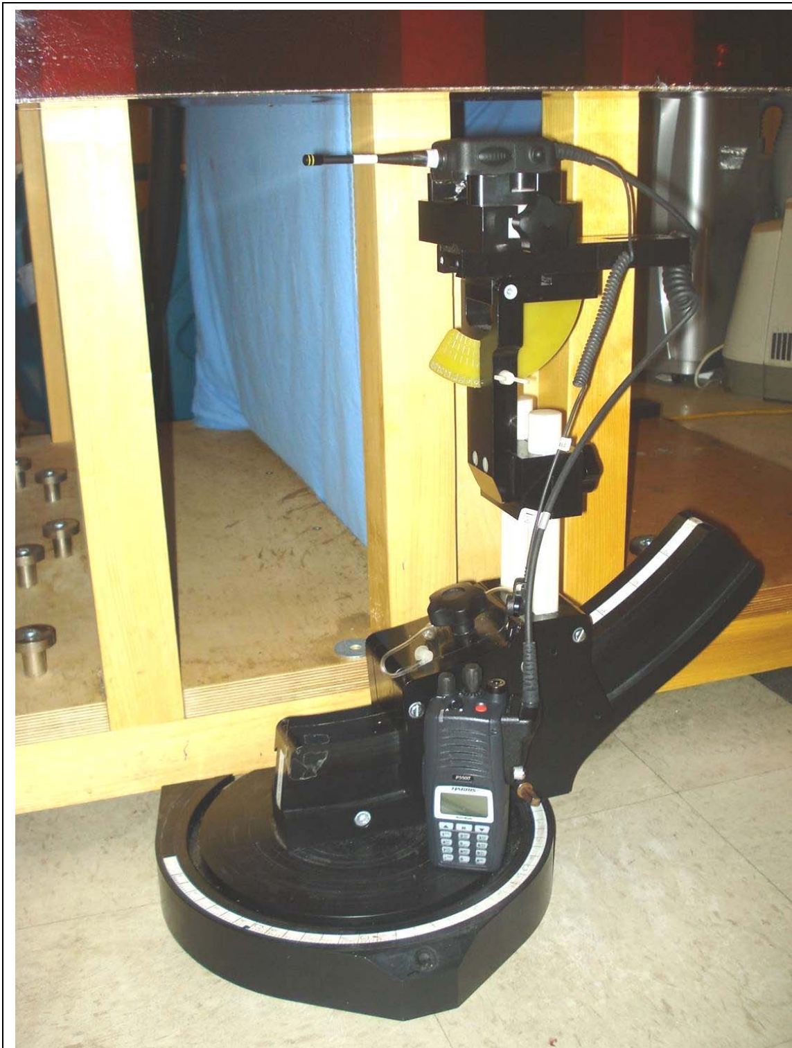
Speaker-mic with Antenna (MC-023933-002) Face Held Test Setup Configuration
