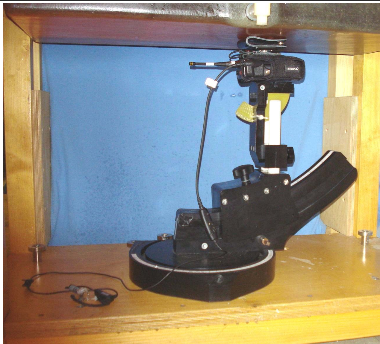
Body Worn Test Setup - Explorer Headset (EA-009580-007), Case (CC-014534-002), Antenna (KRE1011223/01)
