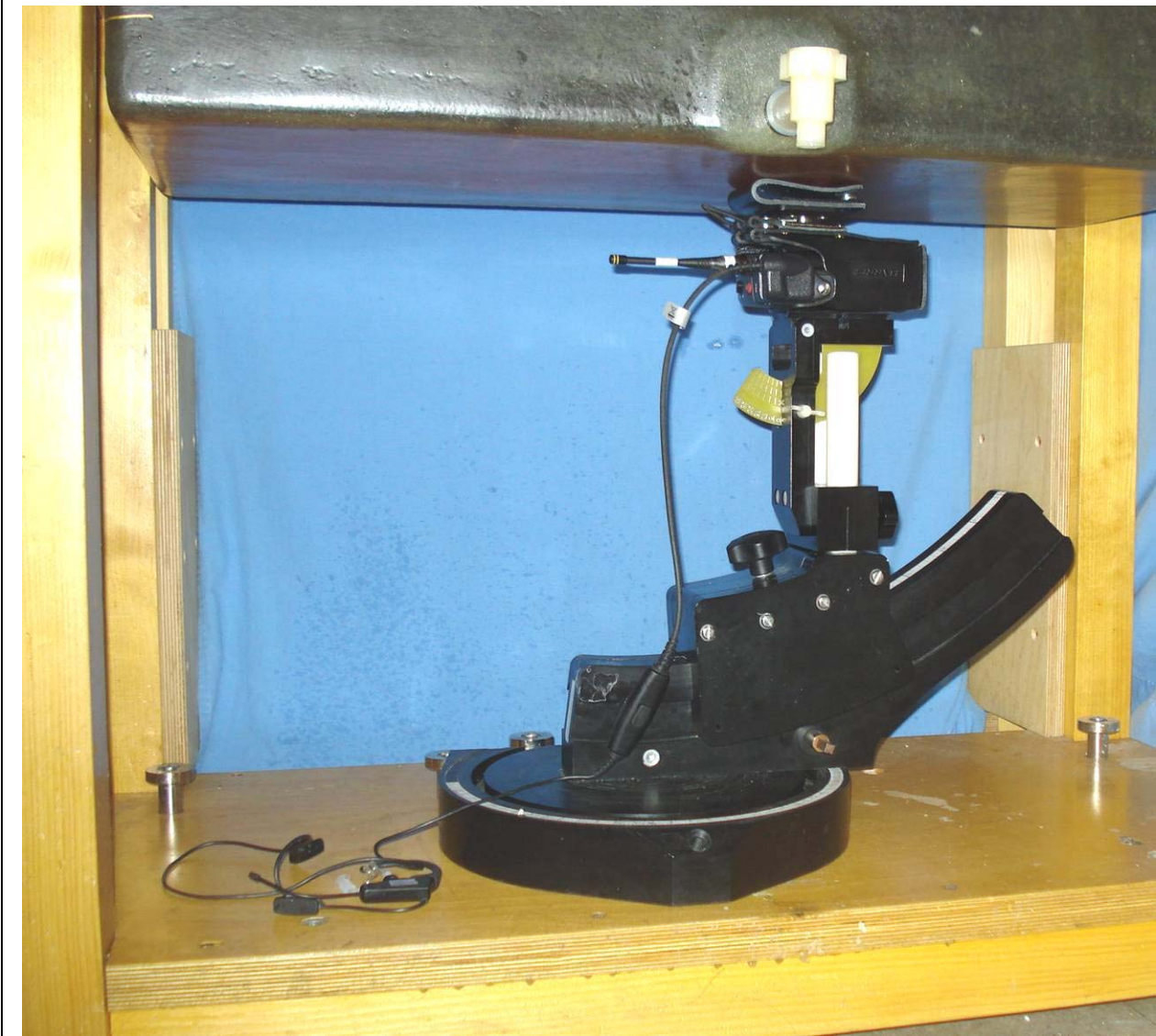
Body Worn Test Setup - Explorer Headset (EA-009580-007), Case (CC-014528-003), Antenna (KRE1011223/01)
