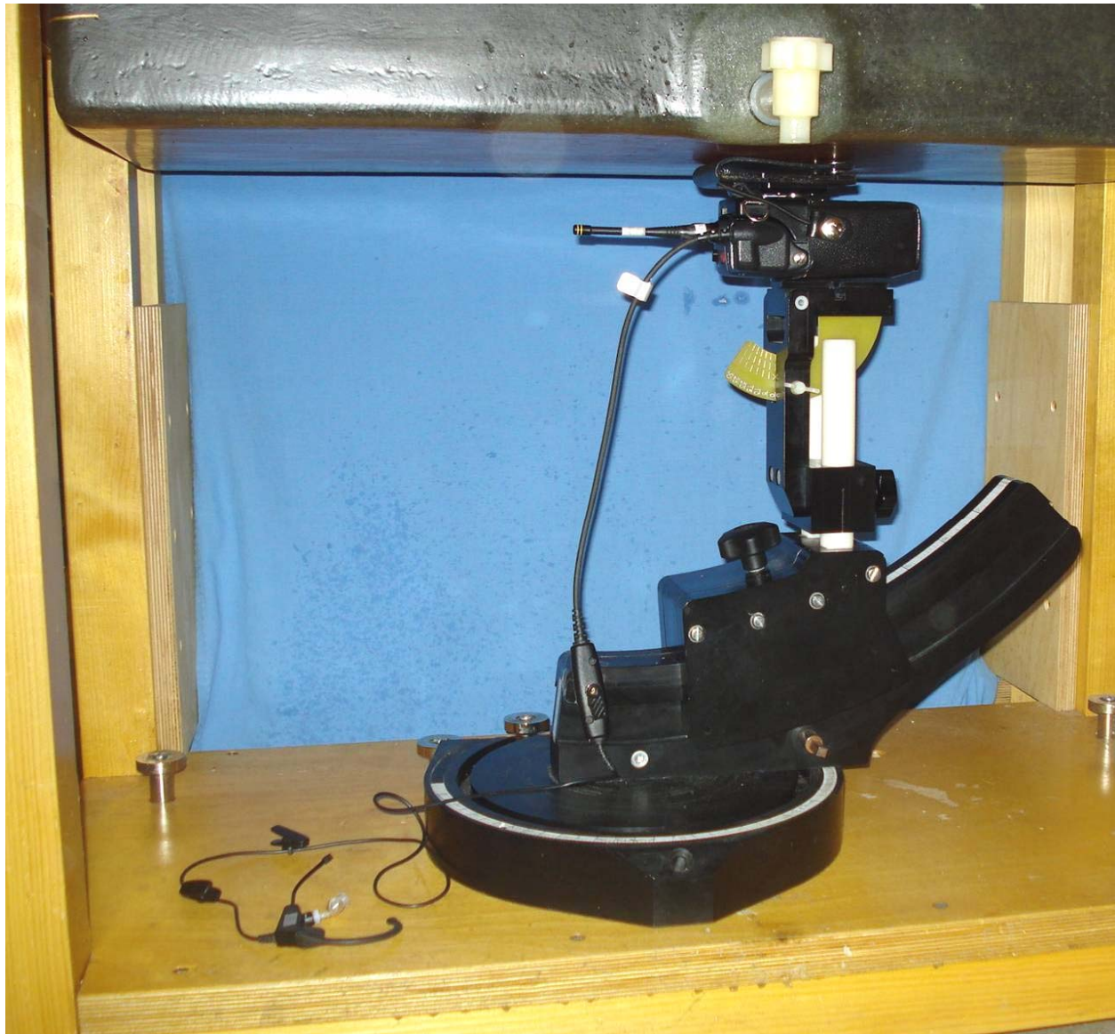
Body Worn Test Setup - Explorer Headset (EA-009580-007), Case (CC-023931-004), Antenna (KRE1011223/01)
