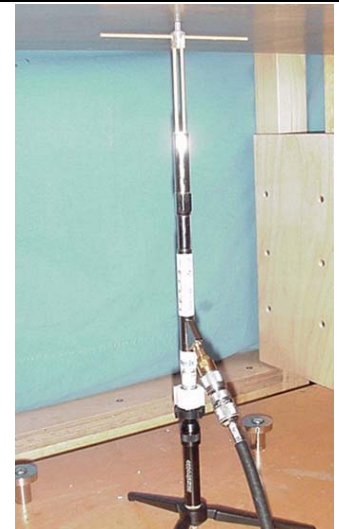
835 MHz SPEAG Validation Dipole Setup
