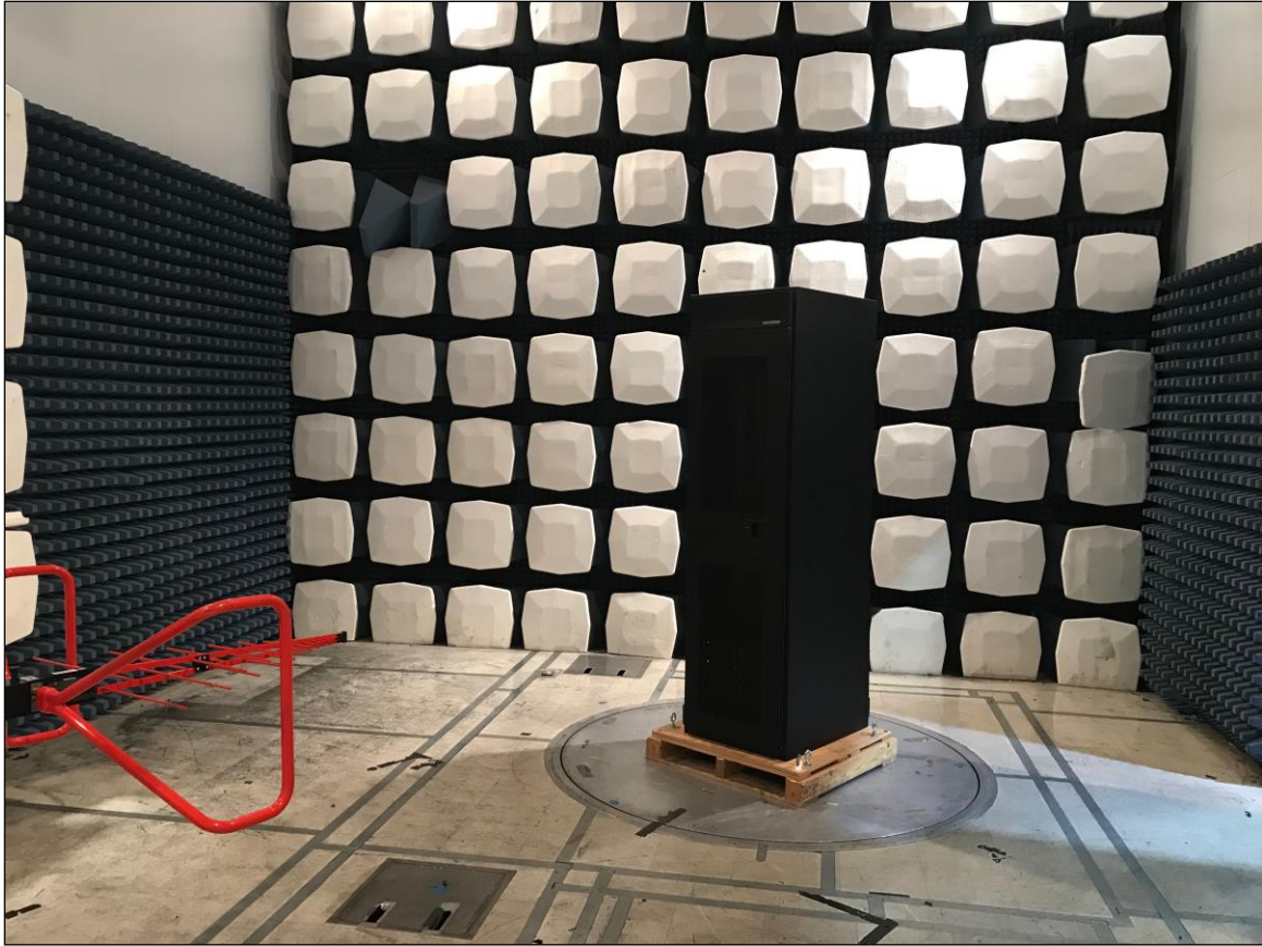
Photograph 1. Radiated Emission Test Setup
