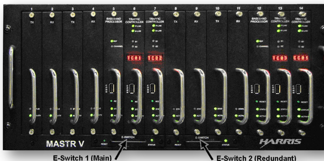
Figure 4-1: MASTR V MHz Base Station Shelf equipped with Four (4) RF Channels
