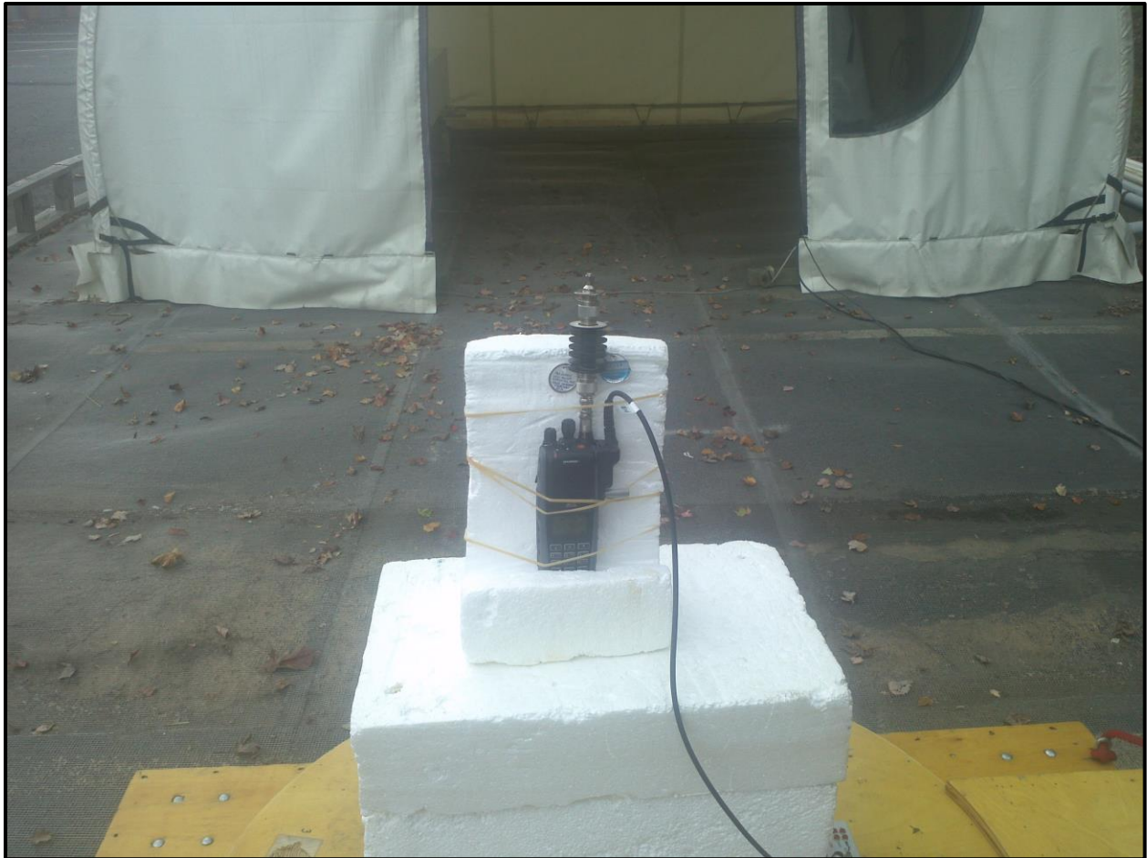
Photograph 1: Radiated TX Spurious Emissions – Front View
