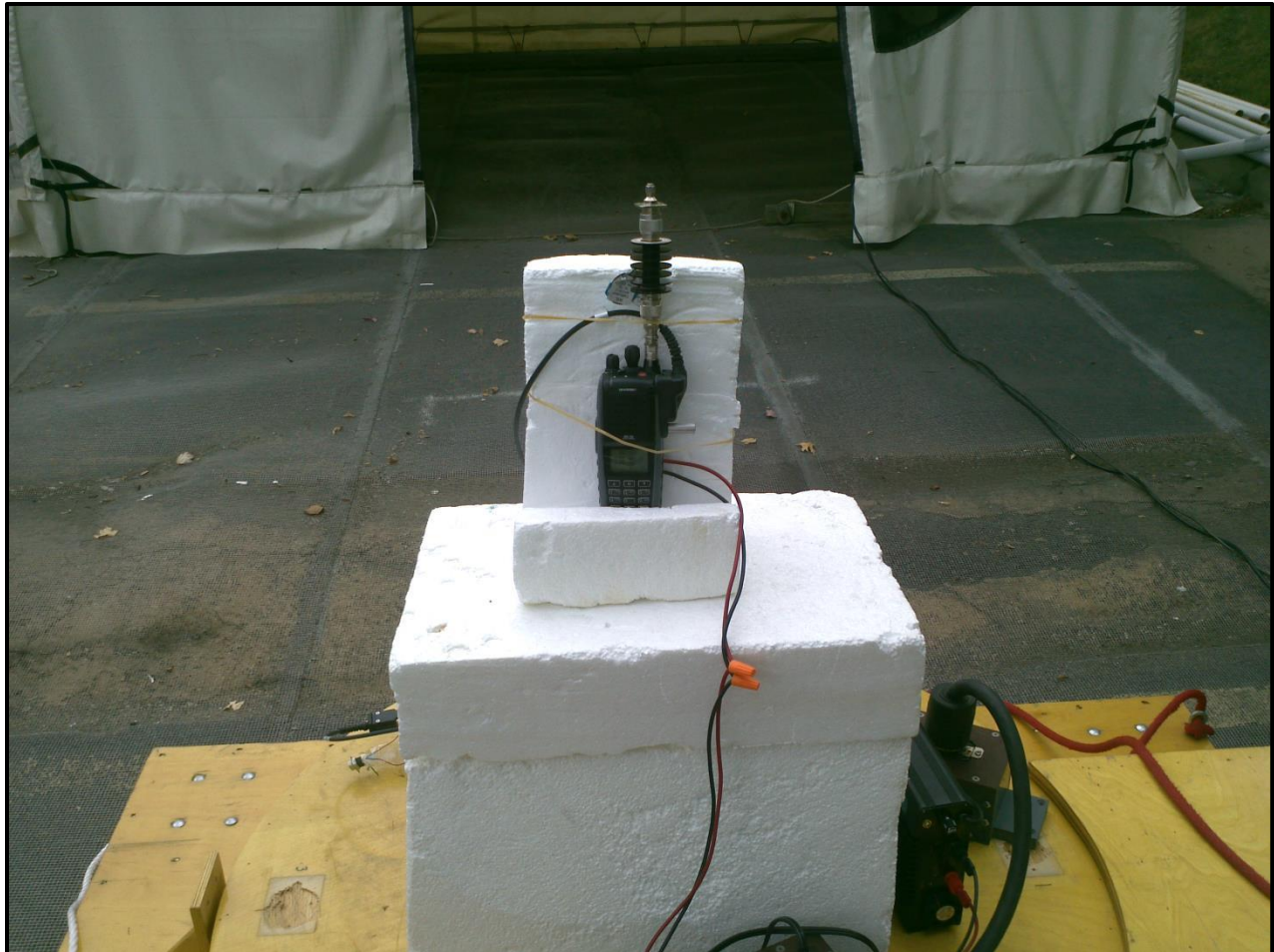
Photograph 1: Radiated TX Spurious Emissions – Front View
