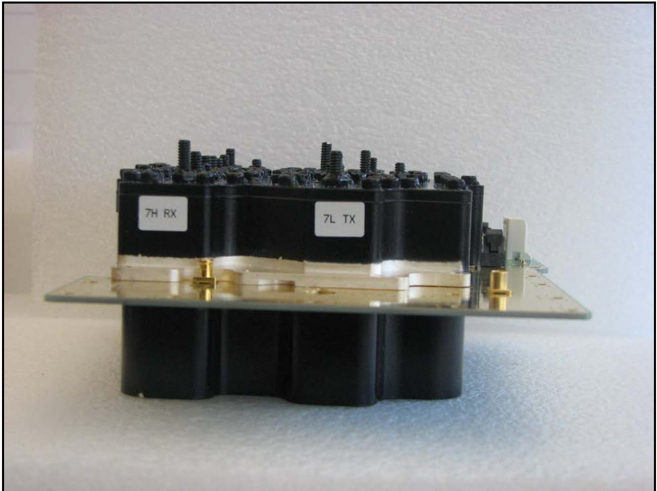
Photograph 24: Dup Filter Side 5
