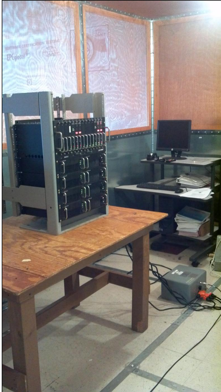
Photograph 1. Conducted Emissions, Test Setup
