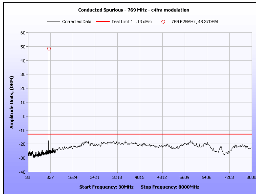
Plot 51. Conducted Spurious Emissions, Channel 769,C4FM
