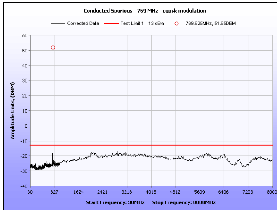
Plot 53. Conducted Spurious Emissions, Channel 769, WCQPSK
