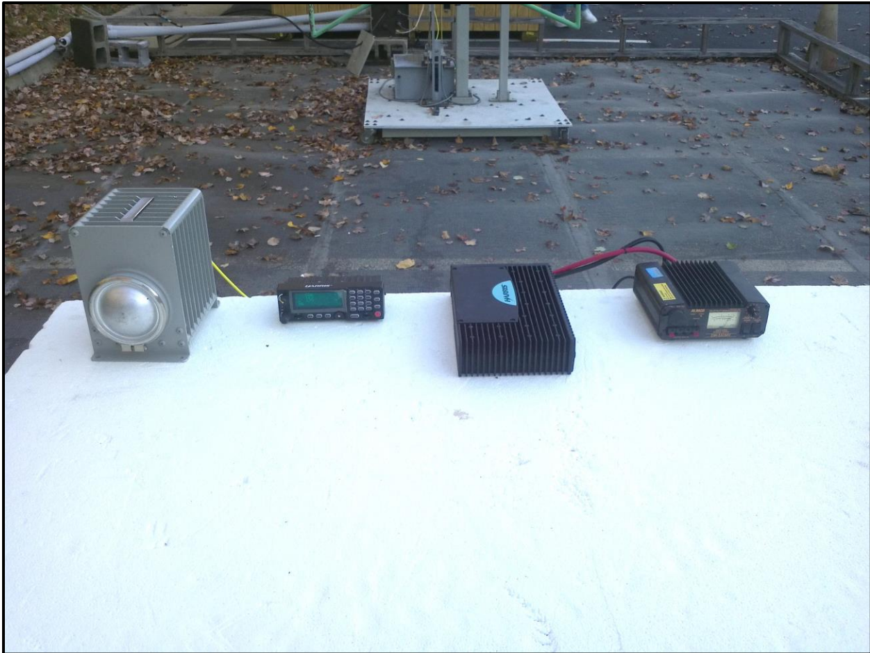
Photograph 1: Radiated TX Spurious Emissions – Front View
