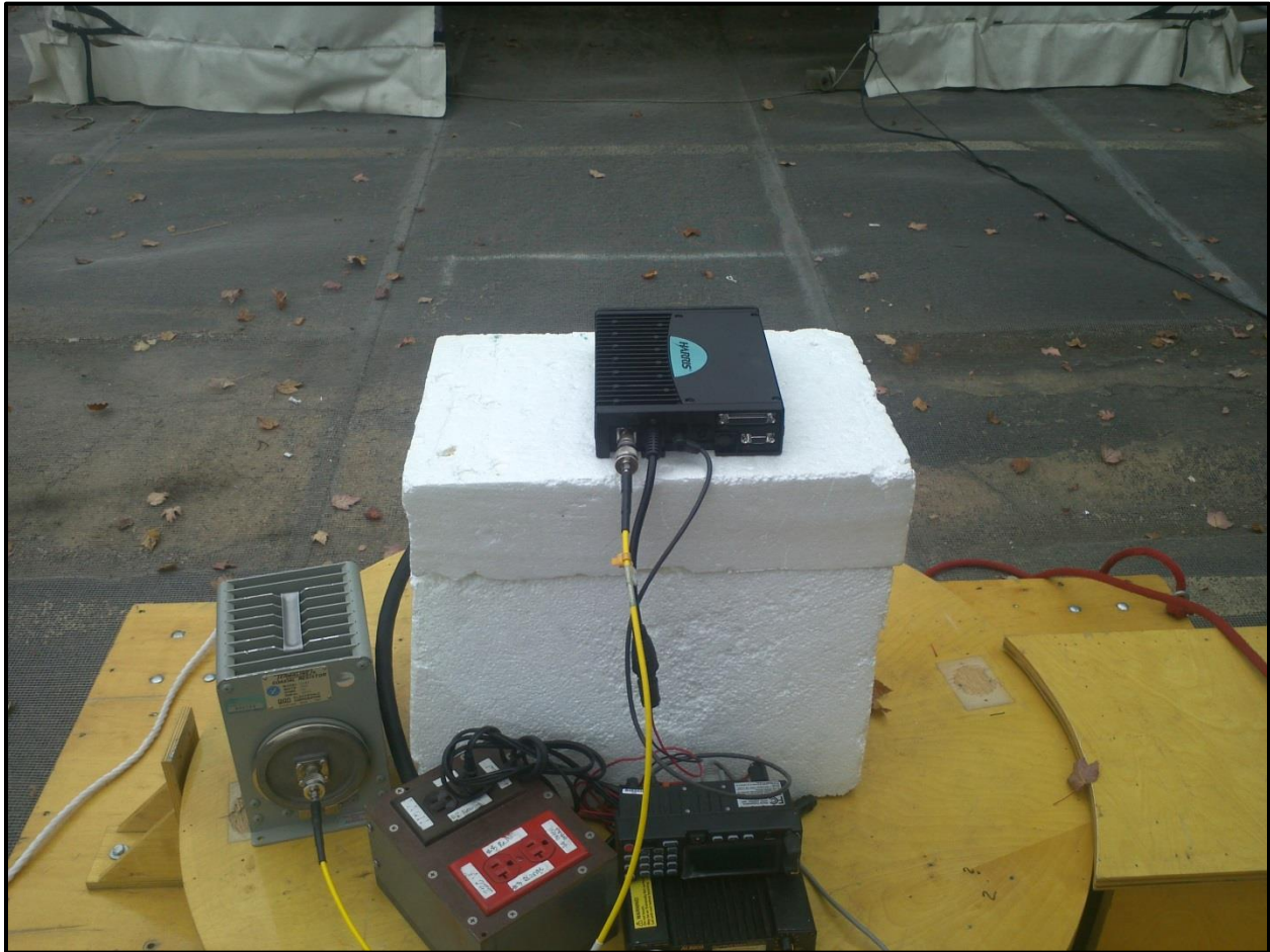
Photograph 2: Radiated TX Spurious Emissions – Rear View
