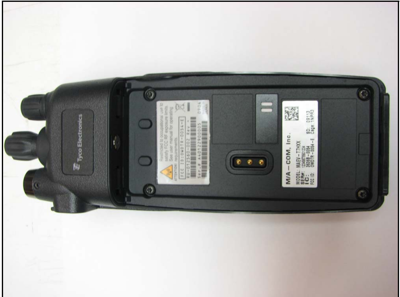
Photograph 3: ID/ RF Label Locations
