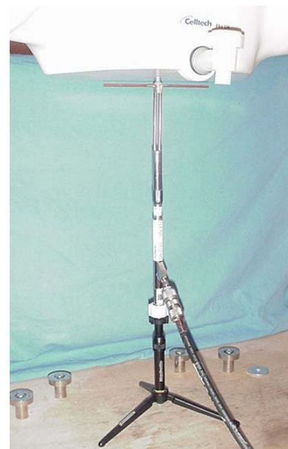
835 MHz Validation Dipole Setup
