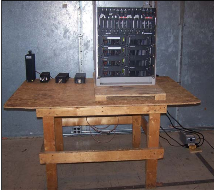
Photograph 1. Conducted Emissions, Test Setup
