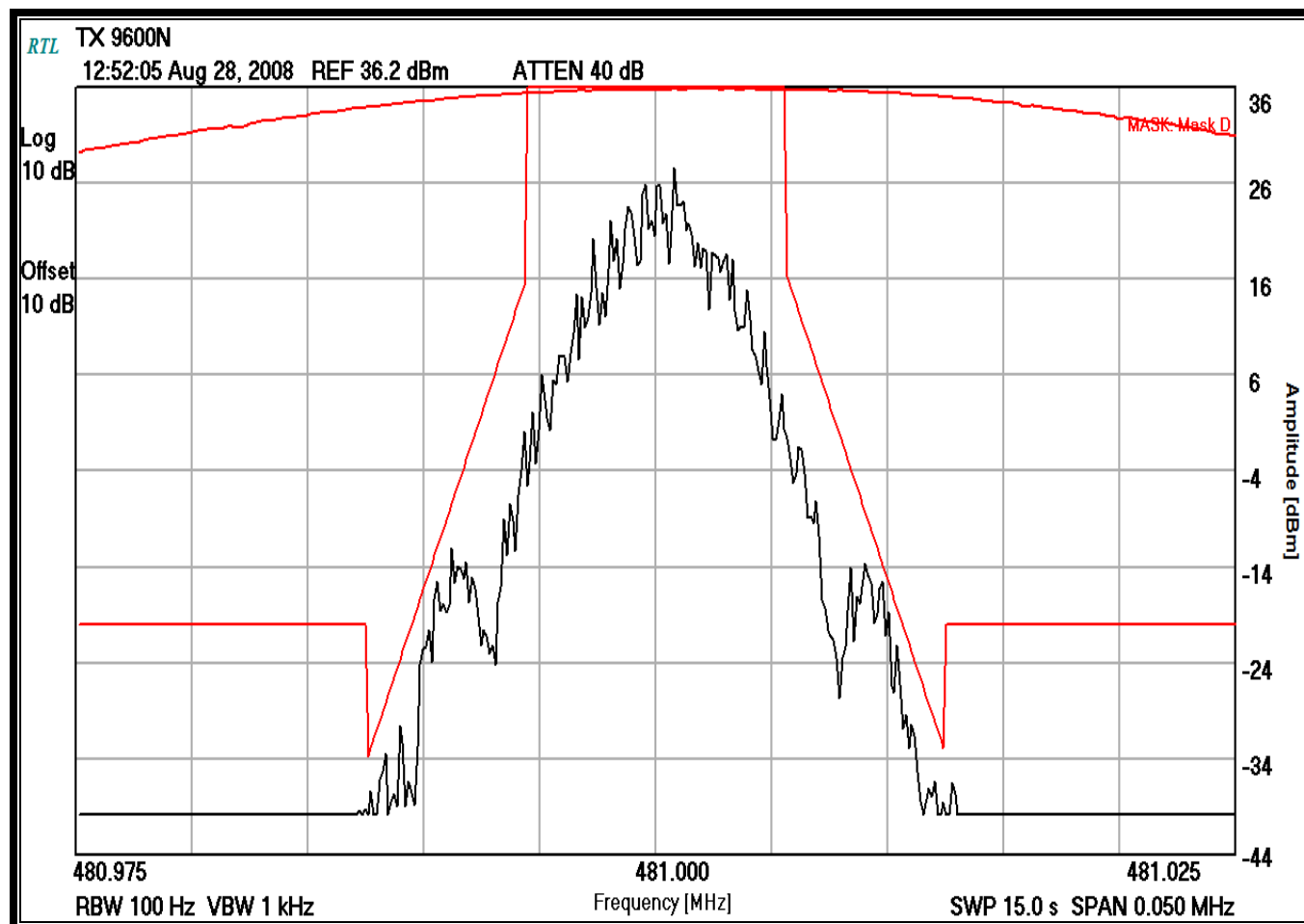
Plot 7-4: Occupied Bandwidth – 481 MHz; Mask D; NB 2-level FSK; 9600 BPS
