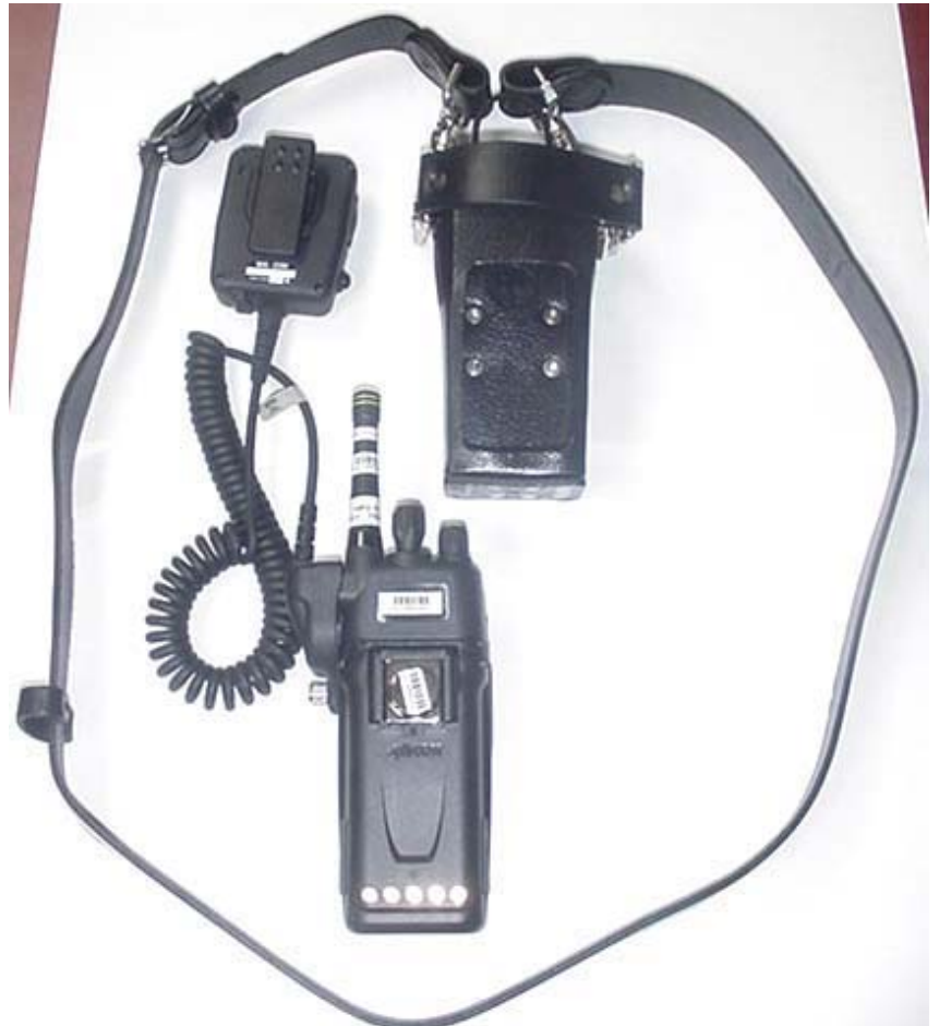
Back of Radio with Swivel Mount (P/N: KRY1011608/2) Leather Case (BEE P/N: FM-016199-004) with shoulder strap D-rings, Shoulder Strap (BEE P/N: CC-014524-001), Short Leather Retaining Strap (BEE P/N: CC-014524-002) & Speaker-Microphone
