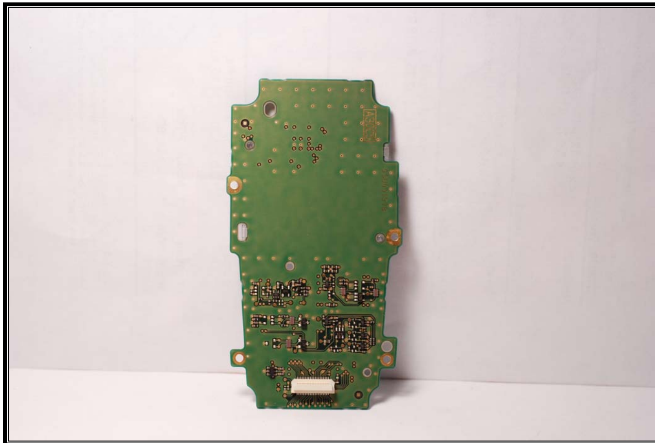
Photograph 17: P7300 Interface PWB Component Side
