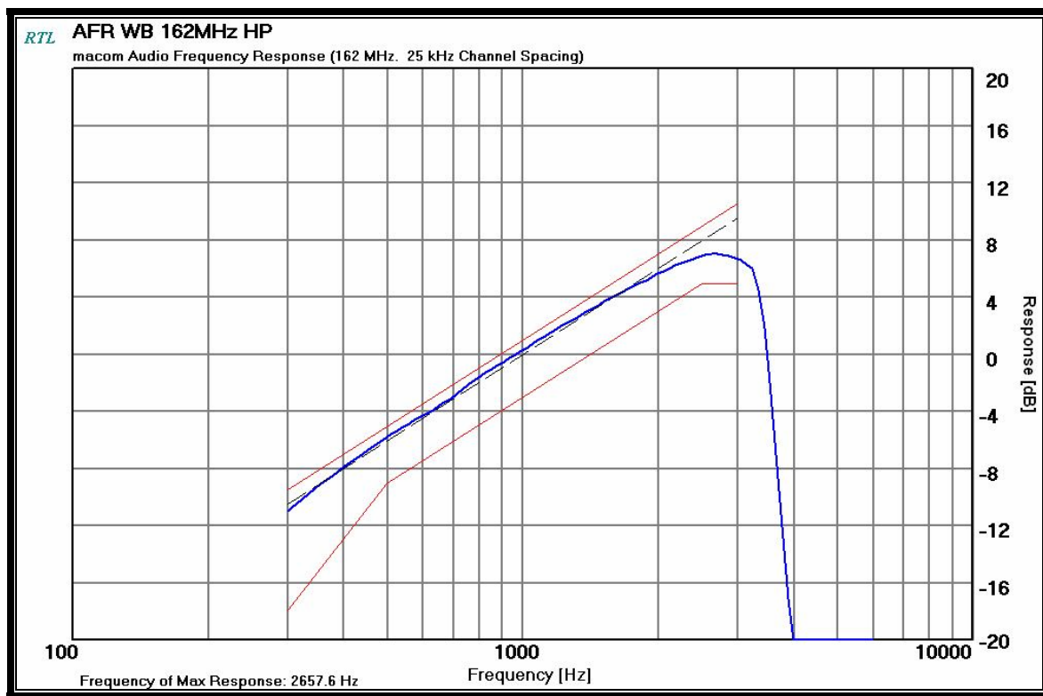
Plot 9-1: Modulation Characteristics - Audio Frequency Response – 162 MHz
