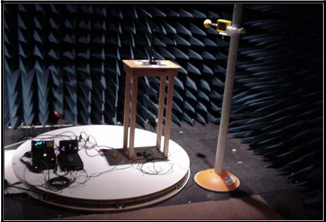
Photograph 6-1: MPE Test Setup for the GPS/900 MHz Antenna in the Elevated Base
