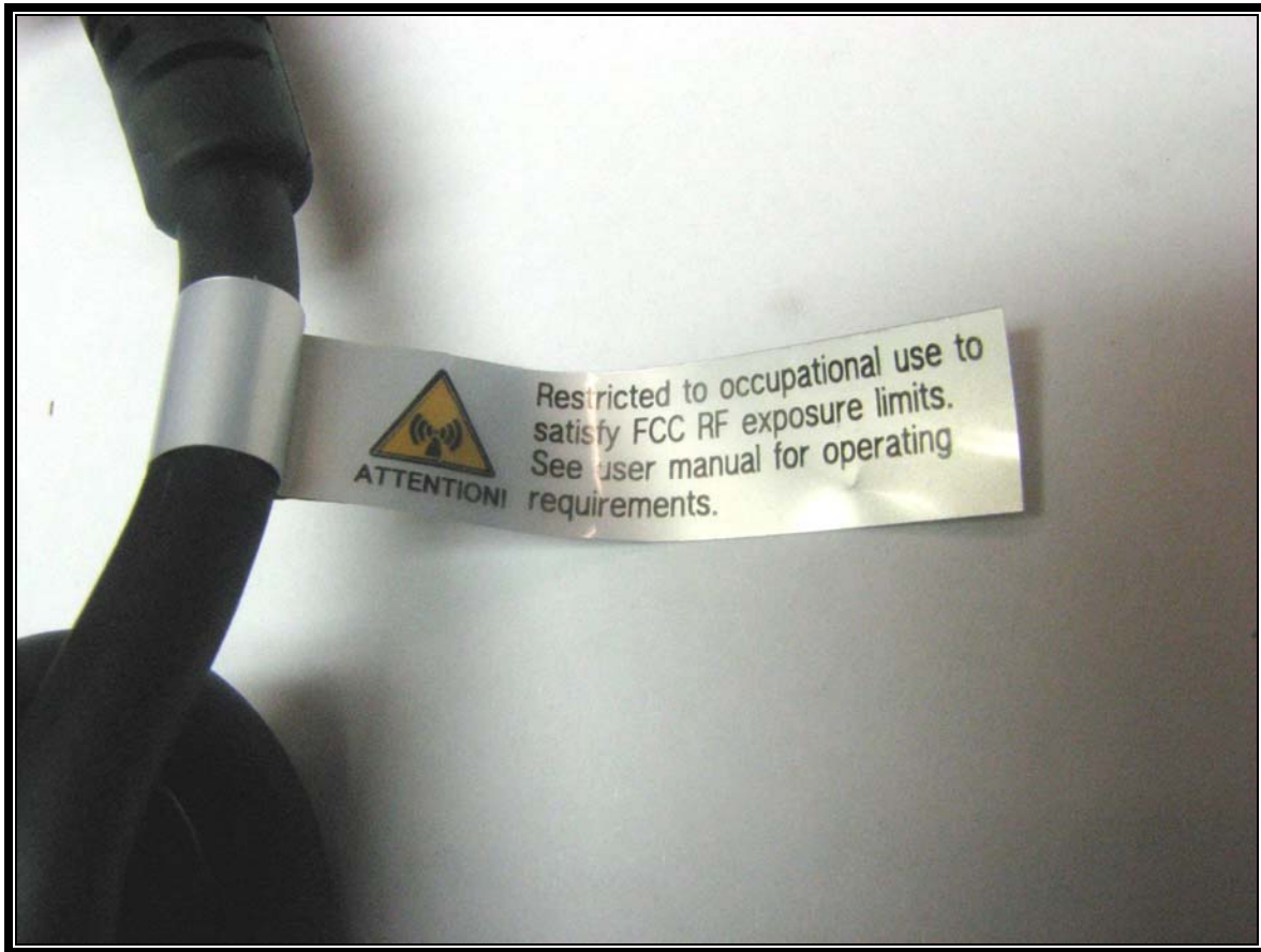
Photograph 5: RF Warning Label on Microphone
